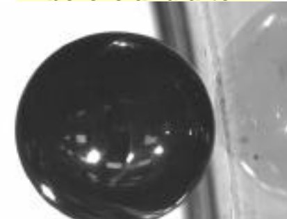
600 Å Pd on PAMS shell - before and after
