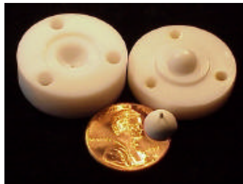
4 mm diameter hemishell ~100 mg/cc, 400 \mu\text{m} wall
