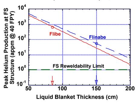
Innermost shield layer/nozzles/feeding tubes cannot be re-welded at any time during operation.
