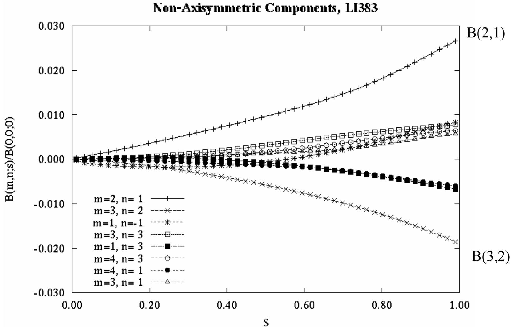
Eight Fourier harmonics with largest amplitude in the N3AEC magnetic spectrum. Note the prominent role of the primary mirror and helical terms. The largest components B(2,1) and B(3,2) have essentially the same magnitude as those in LI383.
