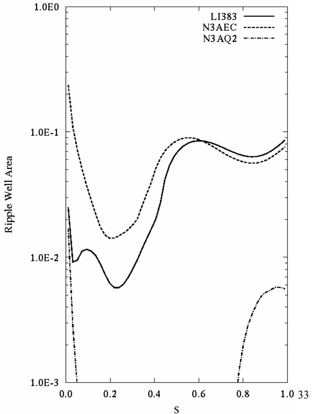
D.3. The effective ripple of N3AEC is about 20% smaller for  $r/a > 0.7$ , while that of N3AQ2 is x4 better.
