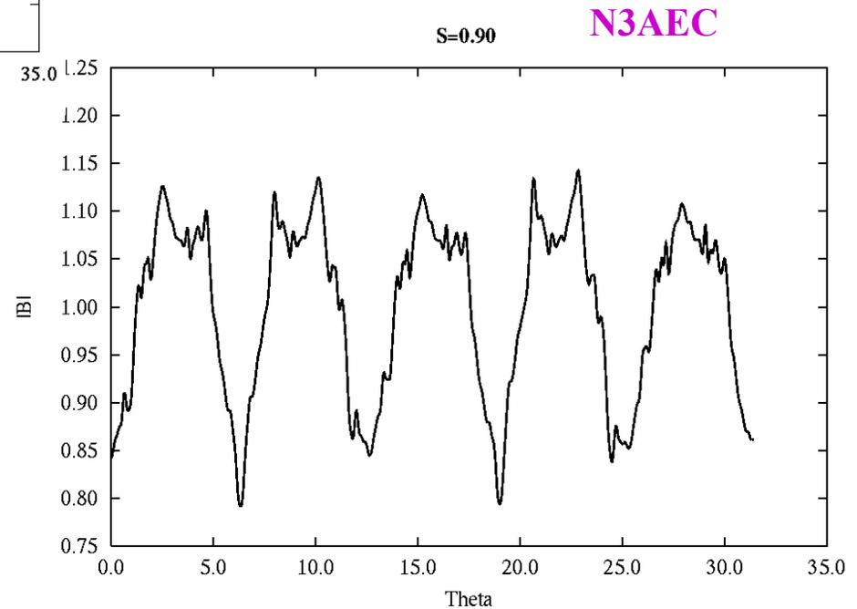
D.5. Comparison of  $\alpha$  loss characteristics: Initial loss in LI383 is much **more** severe than N3AEC. Once the exit time is successfully prolonged in the optimization, the penalty function that minimizes the initial collision-less losses becomes less and less effective.
