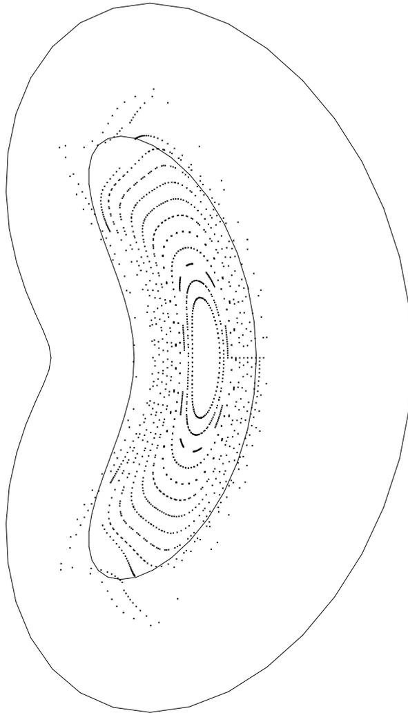
Poincaré section of a line tracing calculation for the MHH2 stellarator displaying the control surface for the coils and the magnetic surfaces at  $\beta = 0$ . There are islands in the scrape-off layer of the solution, where the rotational transform reaches the resonant value  $\iota = 2/5$ . Vertical and toroidal fields have been included to perturb the optimal equilibrium.
