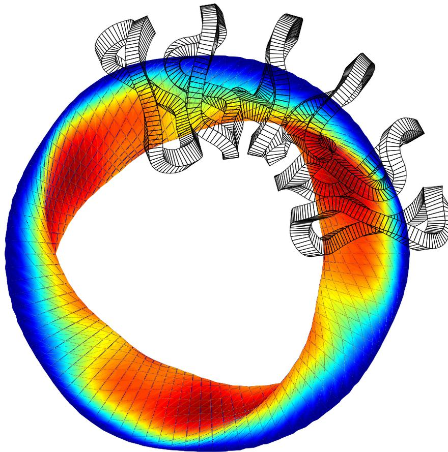
Computational model of fusion plasma in a thermonuclear reactor based on the PG3 simulation of the NCSX experiment. Eighteen moderately twisted modular coils, six of which are plotted, produce a magnetic field whose strength has a symmetry feature displayed by the color map of the plasma surface.
