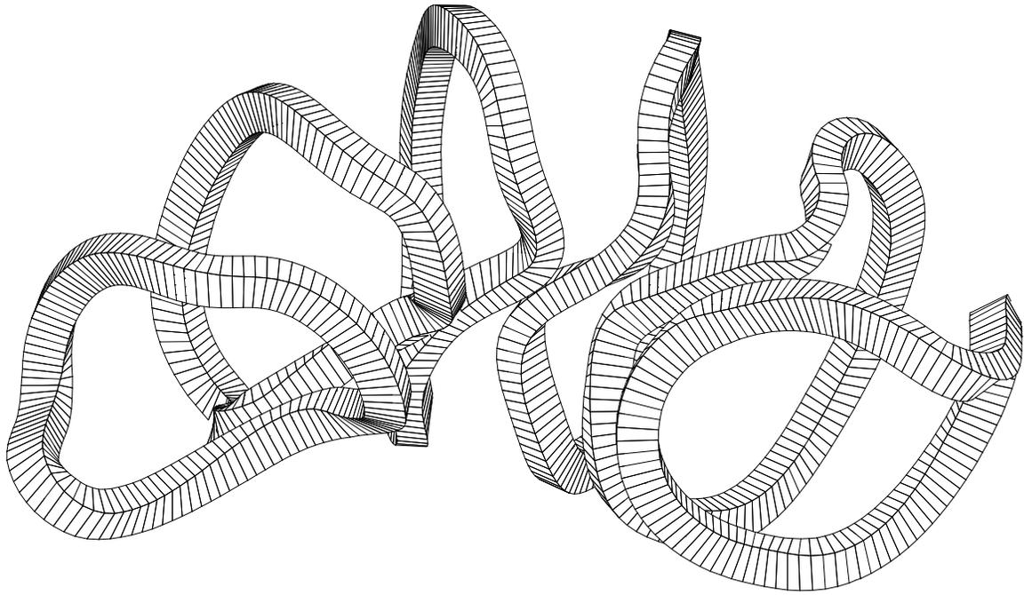
Asymmetric view of six out of twelve modular coils of the MHH2 stellarator in a vacuum magnetic field given by the Biot-Savart law. Judicious filtering of the Fourier series used to calculate filaments specifying the geometry of the configuration defines shapes that are not excessively twisted. Parameters have been adjusted to provide ample space around each coil, and the aspect ratio of the plasma is 3.5.
