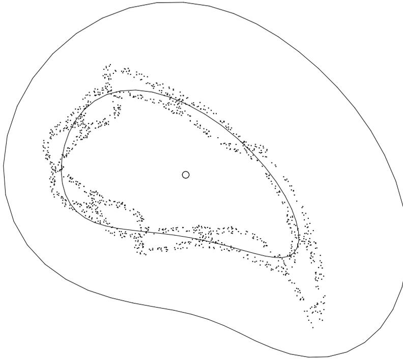
Poincaré section of a free boundary calculation for the MHH2 stellarator displaying the control surface for the coils, the known shape of the plasma at  $\beta = 0$ , a filament that simulates current in the plasma, and magnetic lines computed at finite  $\beta$  in the scrape-off layer of the solution, where the rotational transform is crossing the resonant value  $\iota = 2/5$ .
