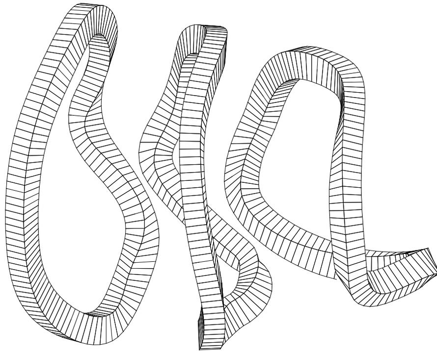
Exterior view of a triad of distinct coils for the MHH2 reactor showing that they are only moderately twisted and are well separated. Good quality of the coils is found by line tracing calculations to produces robust magnetic surfaces.
