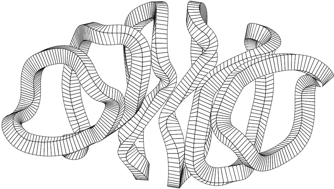
Symmetric view of six out of eighteen modular coils of the PG3 (simulated LI383) stellarator in a vacuum magnetic field given by the Biot-Savart law. Judicious filtering of the Fourier series used to calculate filaments specifying the geometry of the configuration defines shapes that are not excessively twisted and do not introduce superfluous harmonics. The minimum gap between the separatrix and the filaments for the coils is 55% of the plasma radius.
