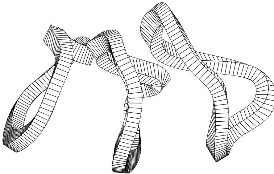
Top view of a triad of distinct coils for the MHH2 reactor showing that there is easy access from outside.
