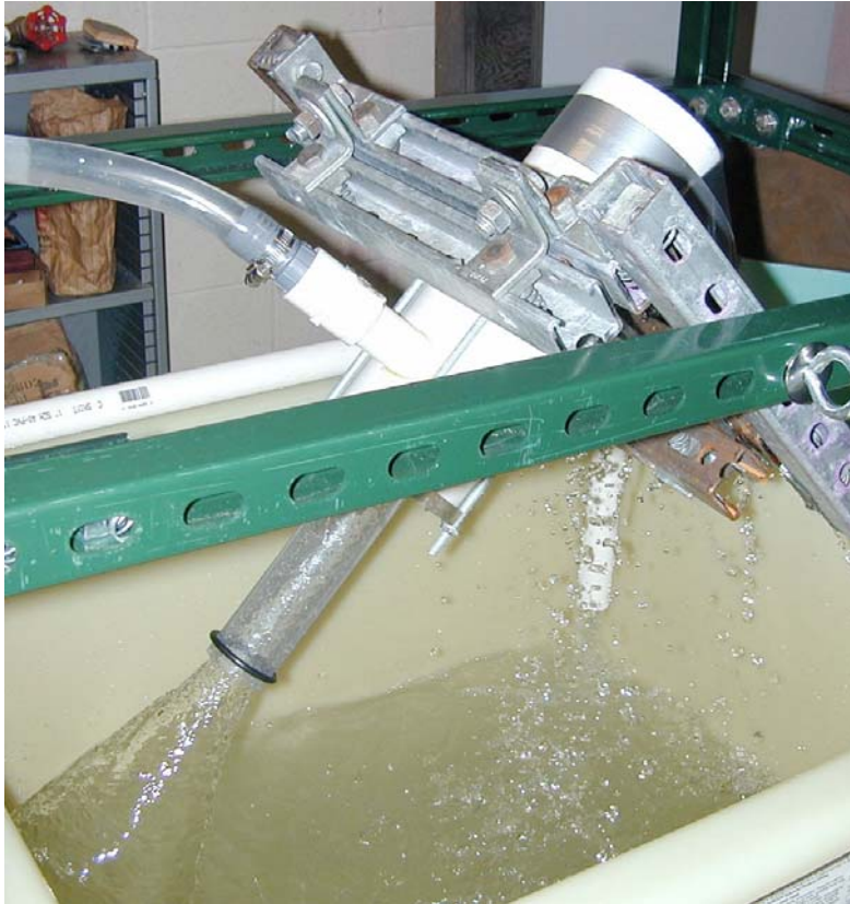
Side view showing operation at 30° angle (extraction nozzle used on right, vortex fan on left)
