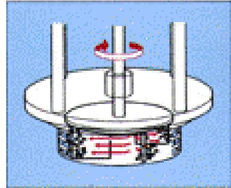
**Powder and fluid thrown outward and milled with high speed blades**
