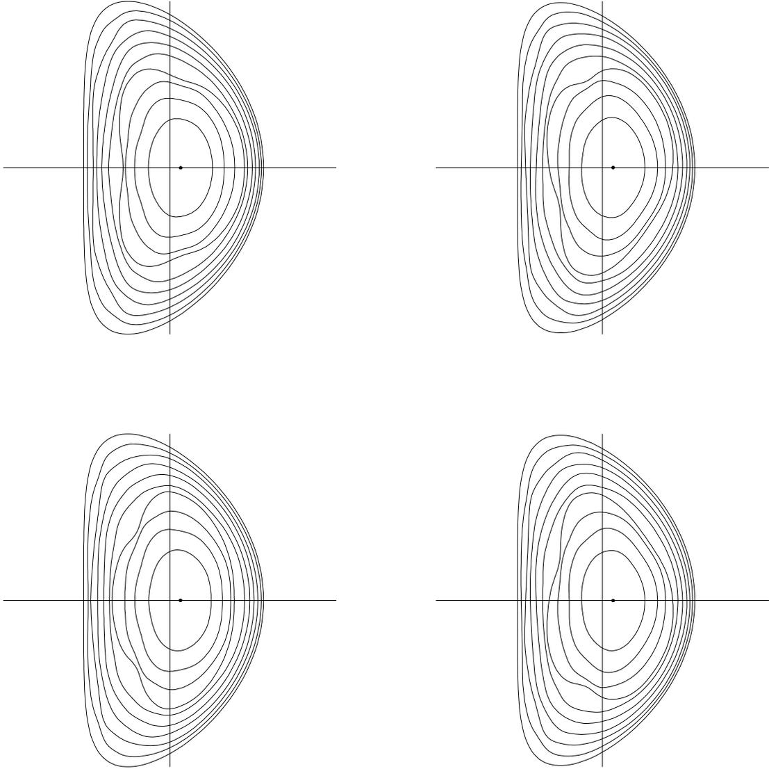
Four cross sections of the flux surfaces over half the torus of a bifurcated ITER equilibrium at  $\beta = 0.05$  with  $p = p_0(1 - s^{1.1})^{1.1}$  and with net current bringing the rotational transform into the interval  $0.9 > \iota > 0.3$ . There is a large  $m = 3$ ,  $n = 2$  magnetic island at  $\iota = 2/3$  in the solution. The calculation suggests that this advanced tokamak reactor is dangerously close to being nonlinearly unstable.
