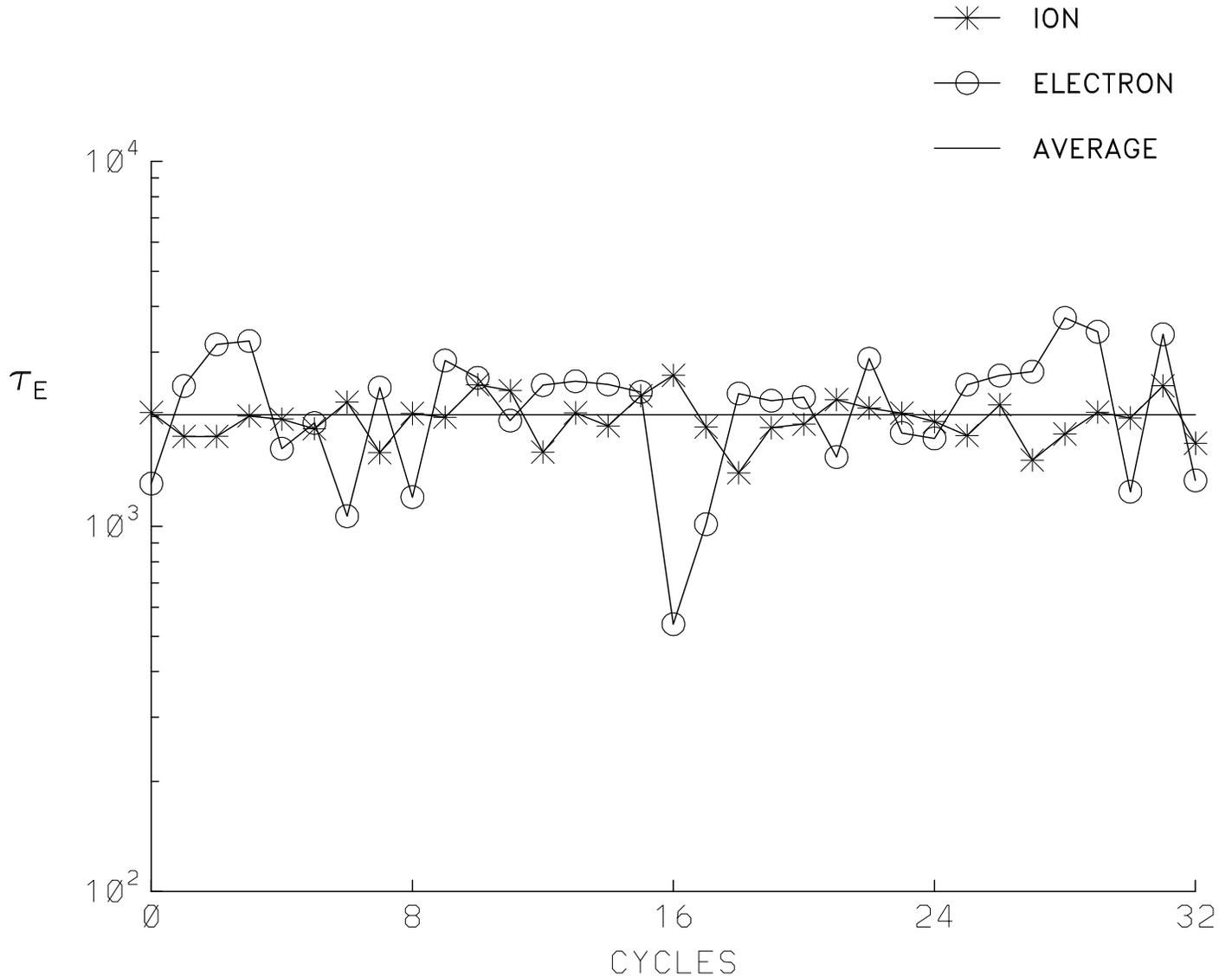
Iterations to quasineutrality in a Monte Carlo computation of the energy confinement time  $\tau_E$ , measured in milliseconds, for an MHH2 reactor with major radius 7 m and plasma radius 2 m at efficient conditions with average  $T = 20$  keV,  $n = 1.4 \times 10^{14} \text{ cm}^{-3}$ , and  $B = 6$  T . The magnetic spectrum has excellent quasi-axial symmetry, and the radial electric field rises to a potential level twice as big as the temperature.
