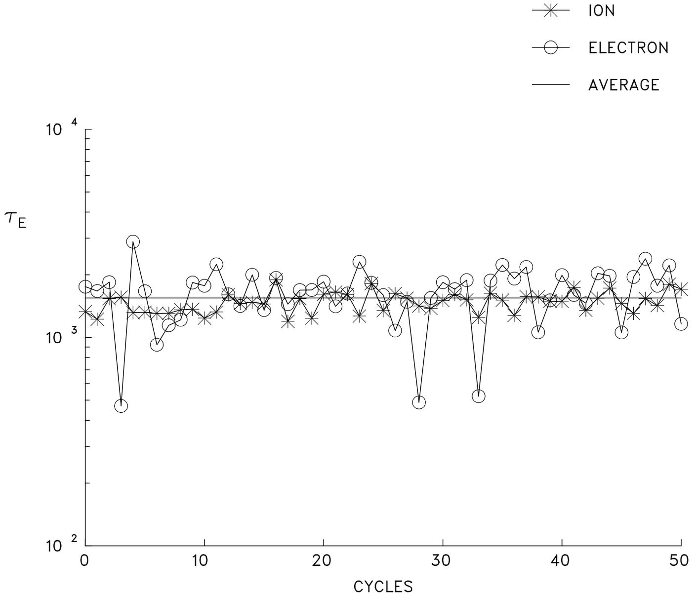
Iterations to quasineutrality in a Monte Carlo computation of the energy confinement time  $\tau_E$ , measured in milliseconds, for a KG3 reactor with major radius 7.2 m and plasma radius 1.6 m at conditions with average  $T = 15$  keV,  $n = 2 \times 10^{14} \text{ cm}^{-3}$ , and  $B = 6.5$  T. The magnetic spectrum has good quasiaxial symmetry, and the radial electric field rises to a potential level twice as big as the temperature.
