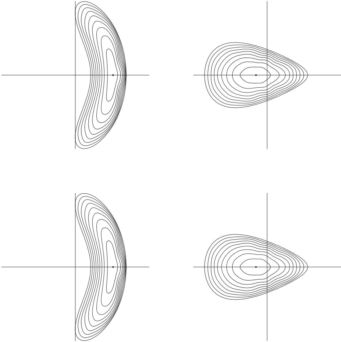
Four cross sections of the flux surfaces over two field periods of a bifurcated MHH2 equilibrium at average  $\beta = 0.06$  with pressure  $p = p_0(1 - s^{1.1})^{1.1}$  and with net current bringing the rotational transform into the interval  $0.64 > \iota > 0.44$ . A low order ballooning mode appears in the solution, and its structure does not change much when the mesh is refined.
