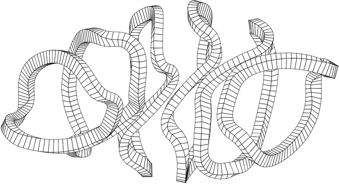
Asymmetric view of 6 out of 18 modular coils for the KG3 stellarator in a vacuum magnetic field given by the Biot-Savart law. Parameters have been adjusted to provide ample space around each coil, and the aspect ratio of the plasma is 4.5. The low number of coils generates significant ripple in the magnetic field. The smallest gap between the separatrix and the filaments defining the coils is two thirds of the plasma radius.
