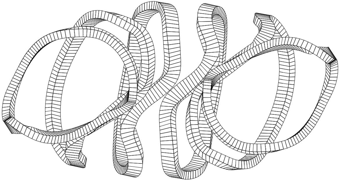
Exterior view of 6 out of 12 modular coils of the MHH2 reactor in a magnetic field given by the Biot-Savart law. There is ample room between each pair of coils to allow for ports to take care of maintenance from the outside, where the geometry is similar to that in a tokamak. At the isolated point where they touch the coils can be separated a little by reshaping them. Smooth coils produce robust flux surfaces that do not deteriorate when changes are made in the vertical and toroidal fields.
