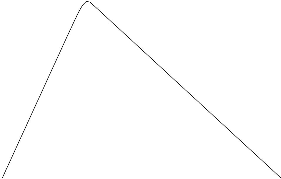
Bad solution for the flux  $\Psi = \Psi(x)$  in the RFP problem using a finite difference scheme that is not in conservation form. If force balance were computed accurately then the two slopes at opposite ends of the curve would have the same size and the apex would be in the middle. The slopes characterize the magnetic field on opposite sides of a current sheet, which is like a chain of magnetic islands.
