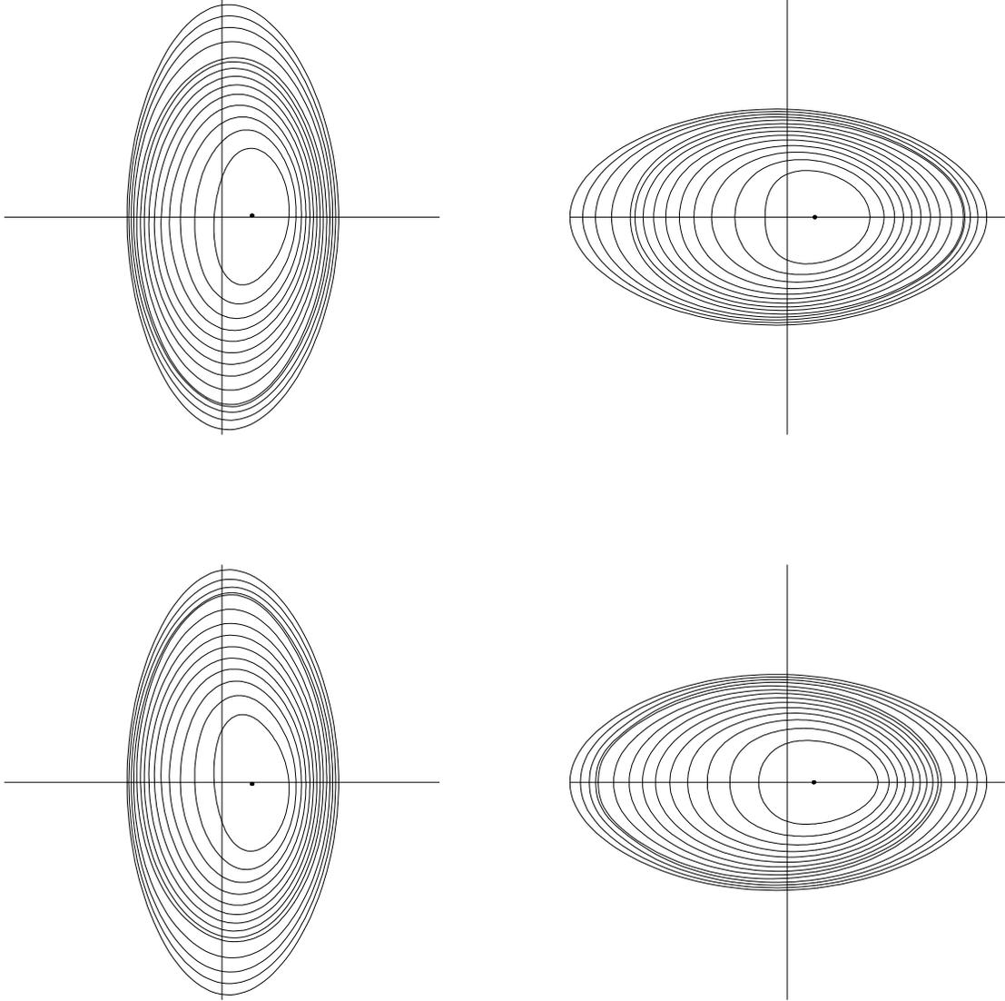
Poincaré map of the flux surfaces at four cross sections over the full torus of a bifurcated LHD equilibrium at  $\beta = 0.032$  with the magnetic axis at a position with plasma radius  $R = 3.6$  m. For a standard pressure profile  $p = p_0(1 - s)$  the global  $m = 1$ ,  $n = 1$  mode of this solution is linearly unstable, but nonlinearly stable. This NSTAB calculation was performed using harmonics of degree up to 24 in the poloidal angle and up to 120 in the toroidal angle.
