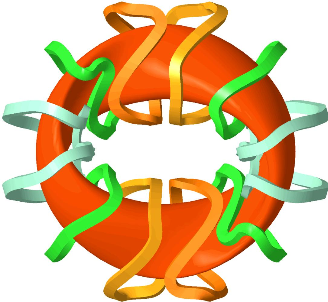
Diagram of an MHH2 stellarator with  $A = 3.5$  designed by running the NSTAB equilibrium code. Twelve moderately twisted modular coils needed to produce the external field are shown. This configuration is a candidate for the stellarator reactor study being conducted at UCSD. Maintenance seems to be feasible through ports between each pair of coils. (Courtesy of Tak-Kuen Mau and Tsueren Wang.)
