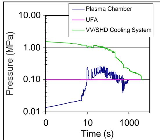
Figure 2. Pressure response to in-vessel LOCA with bypass
