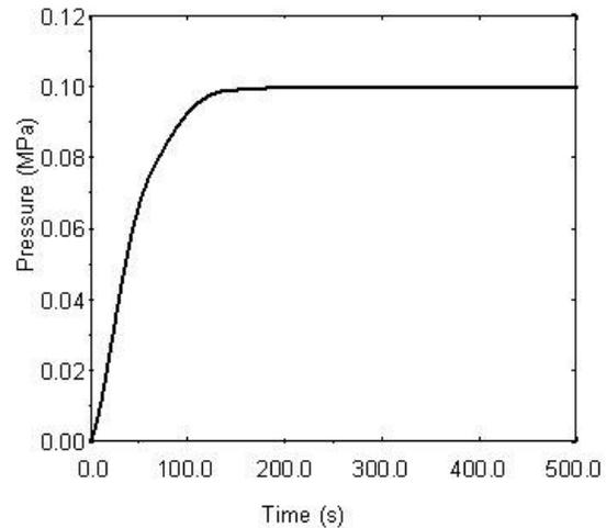
Figure 1. ARIES-AT vacuum vessel pressure during a LOVA.
