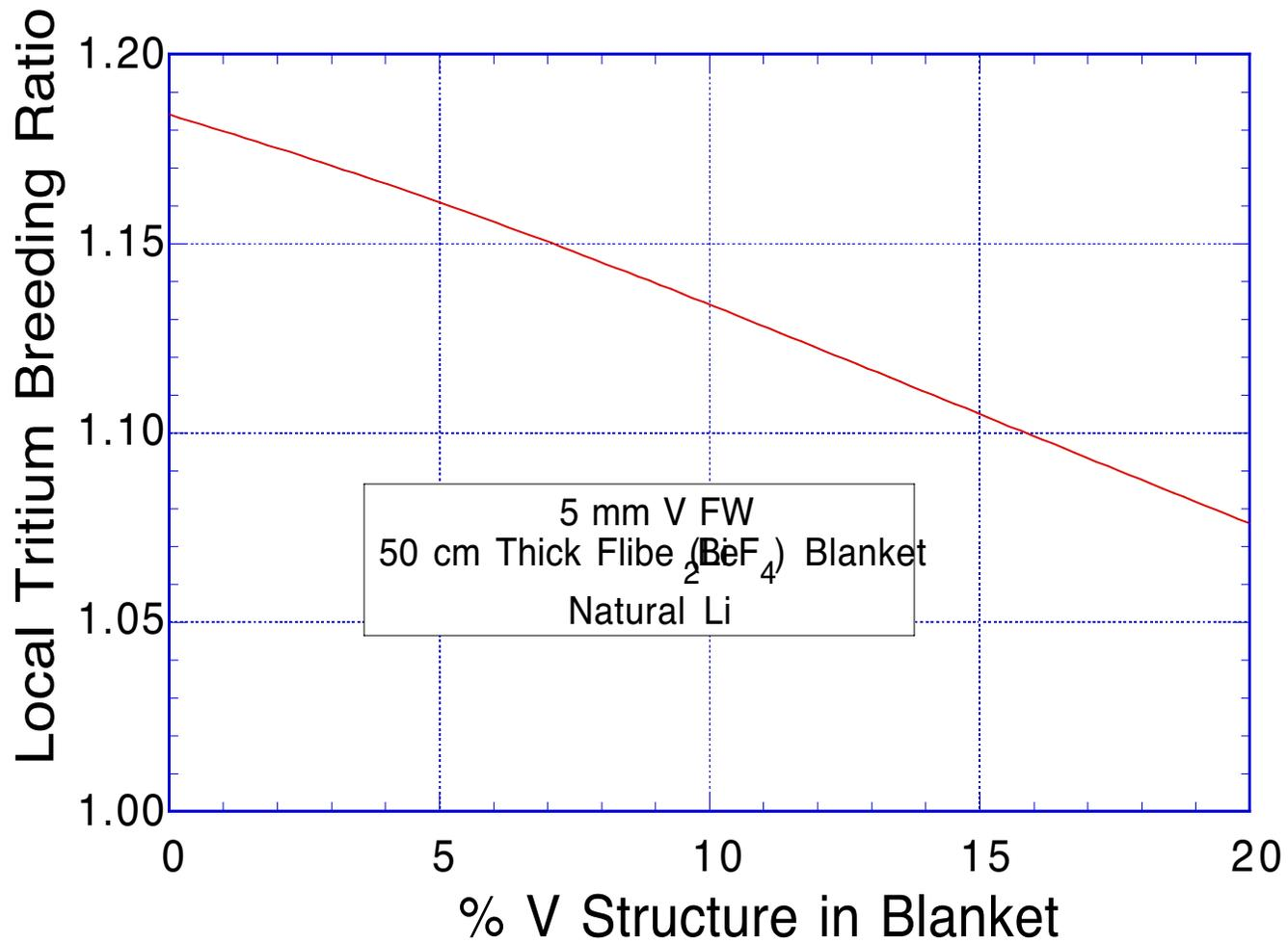
Figure 1. Tritium Breeding Ratio in a Flibe/V Blanket
