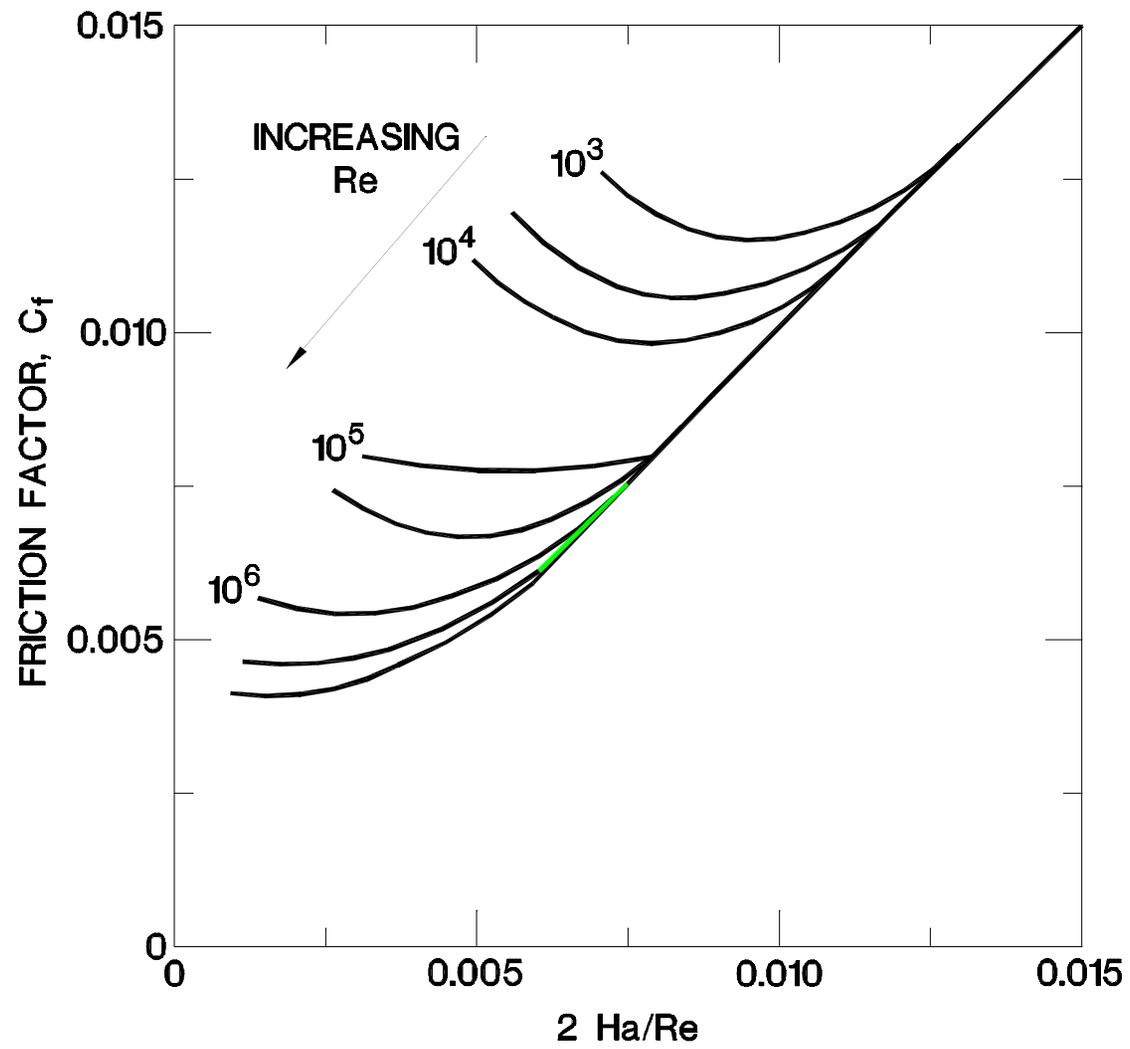
Fig. 4 Effect of MHD on pressure drop.
