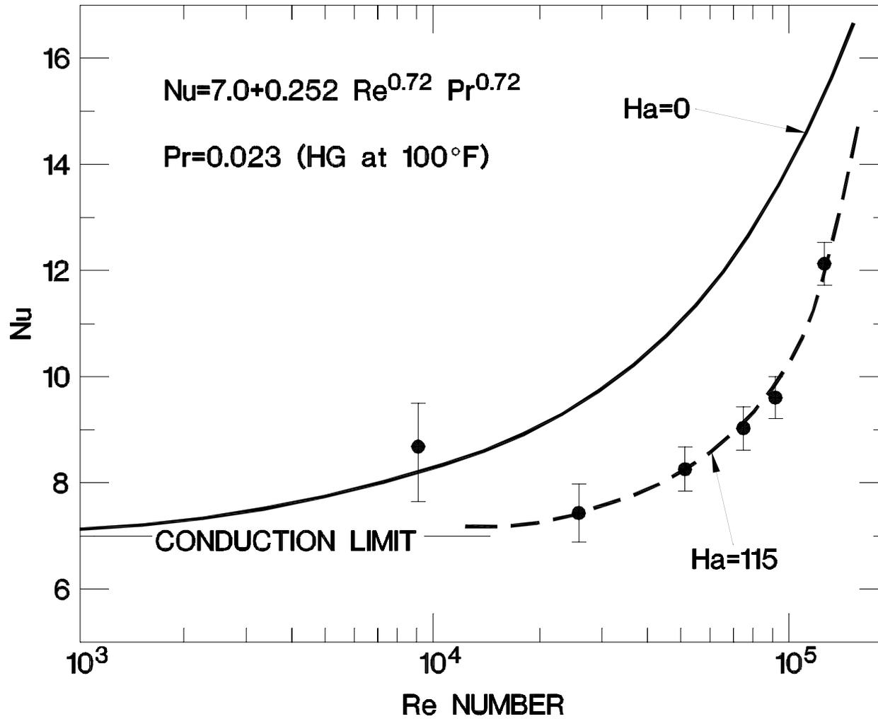
Fig. 5 Effect of MHD on heat transfer.
