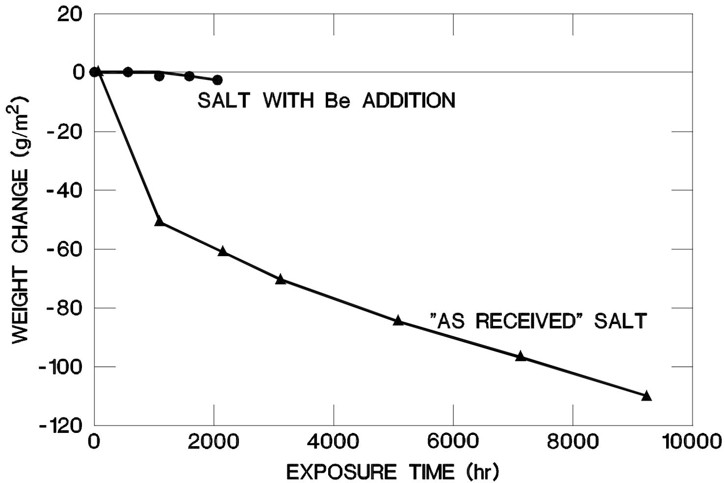
Fig. 3 Weight change versus exposure time for type 316 stainless steel in LiF-BeF<sub>2</sub> salt at the maximum loop temperature of 650 °C.
