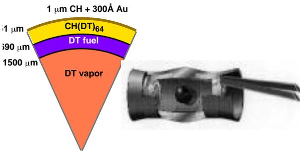
Fig. 1. Baseline direct and indirect drive target designs<sup>5, 6</sup> (not to scale)
