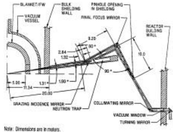
Fig. 7. Layout of final optic<sup>1</sup>
