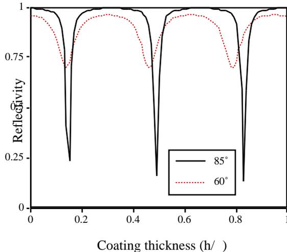
Fig. 8. Effect of surface oxide on Al reflectivity
