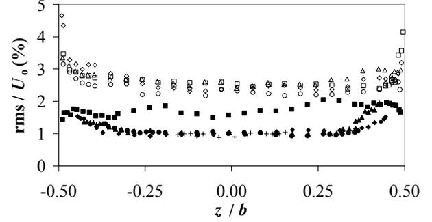
Fig. 4. Normalized profiles of  $u'$  (open) and  $w'$  (closed symbols) for the 1-S configuration at  $Re = 1.2 \times 10^5$  and  $y/\delta = 4.838$  (■), 4.438 (◆), 4.163 (▲), 3.688 (●), and 1.188 (+). Note: Profile at  $y/\delta = 1.188$  for  $w'$  only.
