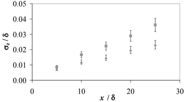
Fig. 6. Graph of  $\sigma_z/\delta$  vs.  $x/\delta$  for 1-S ( $\blacktriangle$ ) and 2-S ( $\blacksquare$ ) flow conditioning configurations at  $Re = 5 \times 10^4$ . The error bars denote 95% confidence intervals.
