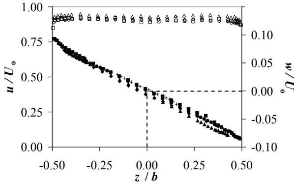
Fig. 3. Normalized profiles of  $u$  (open) and  $w$  (closed symbols) for 1-S configuration at  $Re = 1.2 \times 10^5$  and  $y/\delta = 4.838$  (■), 4.438 (◆), 4.163 (▲), 3.688 (●), and 1.188 (+). Note: Profile at  $y/\delta = 1.188$  for  $w$  only.
