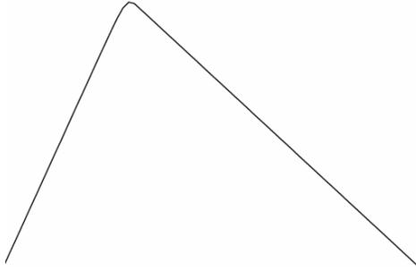
Fig. 1. Bad solution for the flux  $\Psi = \Psi(x)$  in the RFP problem using a finite difference scheme that is not in conservation form. If force balance were computed accurately then the two slopes at opposite ends of the curve would have the same size and the apex would be in the middle. The slopes characterize the magnetic field on opposite sides of a current sheet, which is like a chain of magnetic islands.
