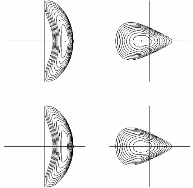
Fig. 2. Four cross sections of the flux surfaces over two field periods of a bifurcated QAS equilibrium at  $\beta = 0.06$  with  $p = p_0(1 - s^{1.1})^{1.1}$  and with net current bringing the rotational transform into the interval  $0.65 > \iota > 0.45$ . A low order ballooning mode appears in the solution, which has an obvious asymmetry.
