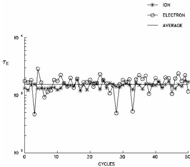
Fig. 3. Iterations to quasineutrality in a Monte Carlo computation of the energy confinement time  $\tau_E$ , measured in milliseconds, for an NCSX configuration with major radius 7.2 m and plasma radius 1.6 m at average  $T = 15$  keV,  $n = 2 \cdot 10^{14} \text{ cm}^{-3}$ , and  $B = 6.5$  T. The magnetic spectrum has good quasiaxial symmetry, and the radial electric field rises to a potential level twice as big as the temperature.
