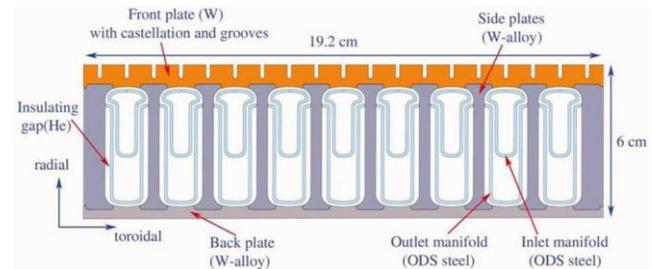
Fig. 1. Cross section of the ARIES divertor.
