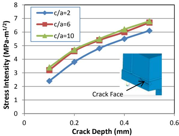
Fig. 7. Stress intensity factors at shutdown for a crack between the tiles.
