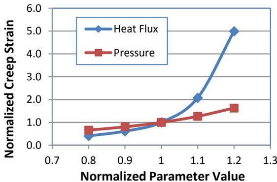
Fig. 12. Normalized variation in peak creep strain for different values of the surface heat flux and coolant pressure. The baseline flux is 6.7 MW/m<sup>2</sup>. The baseline pressure is 10 MPa.
