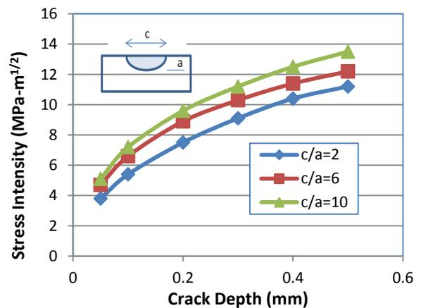
Fig. 5. Stress intensity factor as a function of aspect ratio for a semi-elliptical crack on the inner surface of the divertor. In this plot,  $c$  represents the width of the crack and  $a$  represents the depth.
