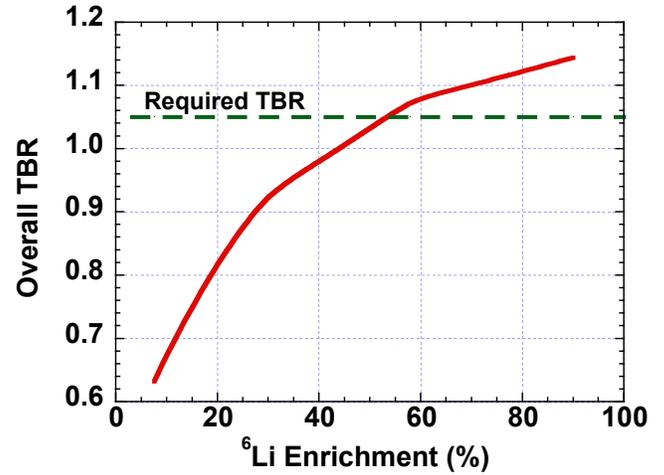
Fig. 6. Sensitivity of TBR to  $^6\text{Li}$  enrichment.
