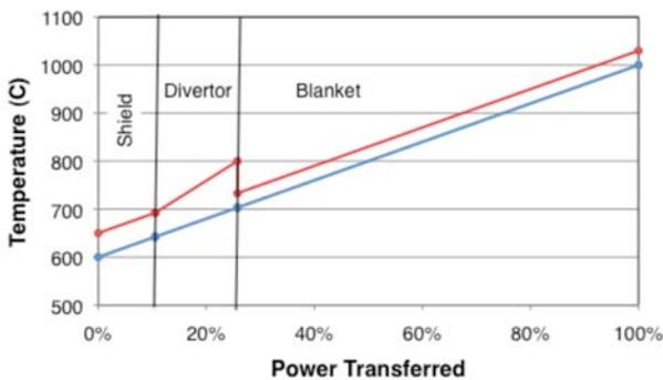
Fig. 11. Thermal power handling in the primary heat exchanger. The top line represents the primary coolant and the bottom line represents the secondary coolant.
