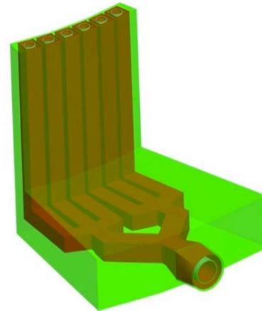
Fig. 7. Inlet manifolding concept for the inner ducts.
