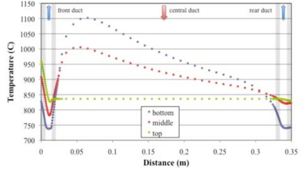
Fig. 9. 2D thermal analysis of the blanket
