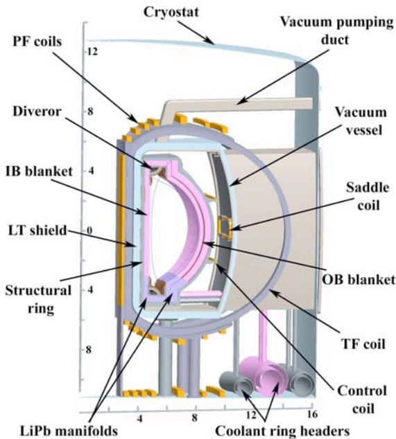
Fig. 1. Cross section of ARIES-ACT1 power core
