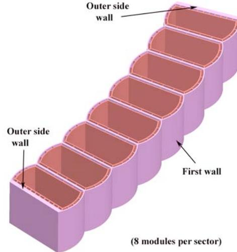
Fig 5. Inboard blanket cross section at midplane
