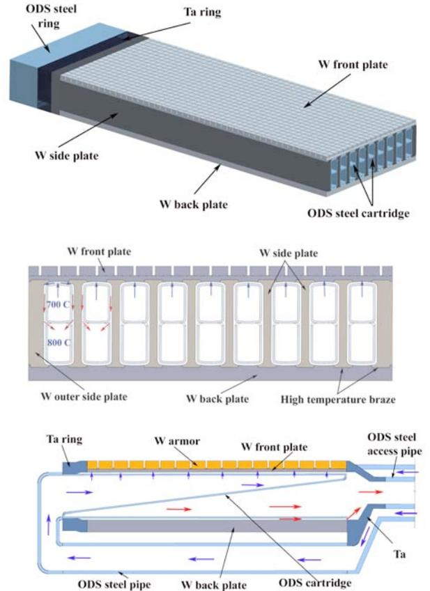
Fig. 4. Drawing of the plate divertor, showing the steel inlet cartridges inserted into the substrate, the castellated armor and the transition joints: a) elevation view, b) cross section, c) flow paths for inlet, outlet and slot jet.
