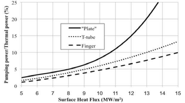
Fig. 3. Comparison of pumping power for the three main divertor concepts (these results were obtained using 600/700 C inlet/outlet temperature).
