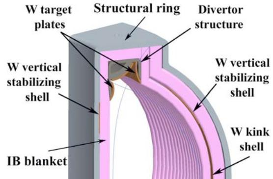
Fig. 2. Details of the replacement unit upper half
