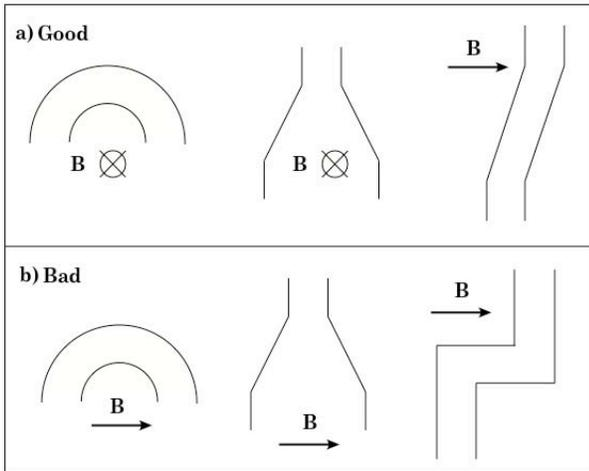
Fig. 6. Design elements that produce (a) small 3D effects or (b) large 3D effects.
