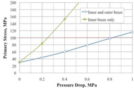
Fig. 10. Pressure stress reduction achieved by brazing the inner and outer blanket pipes
