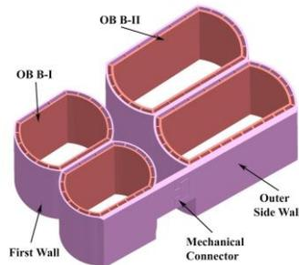
Fig. 4 Configuration of the outboard blanket
