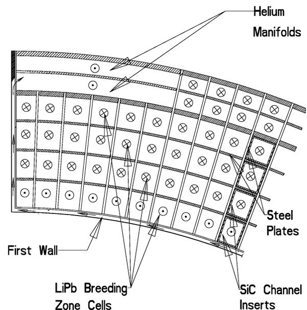
**Fig 2. Cross-section of an ARIES-ST blanket module.**
