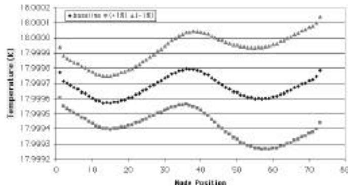
Figure 4. Baseline DT surface temperature distribution and sensitivity to variations in hohlraum material properties.
