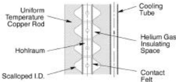
Figure 3. Configuration of the thermal control system
