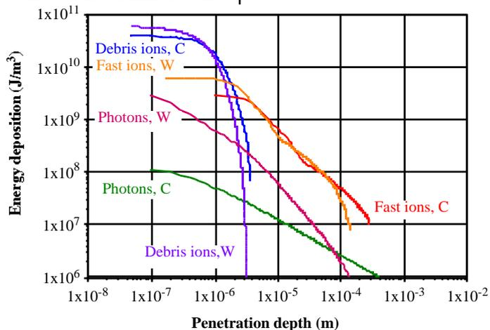
Figure 1 Energy deposition in W and C as a function of penetration depth for DD target x-ray and ion spectra.
