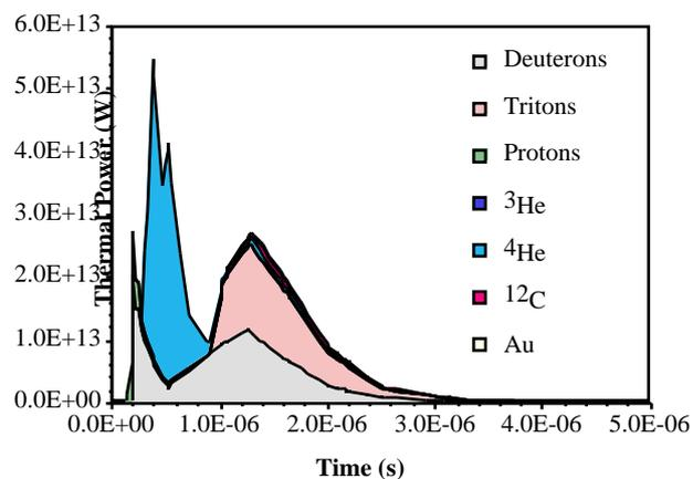
Figure 2 Temporal distribution of ion power at chamber wall for DD target ion spectra.
