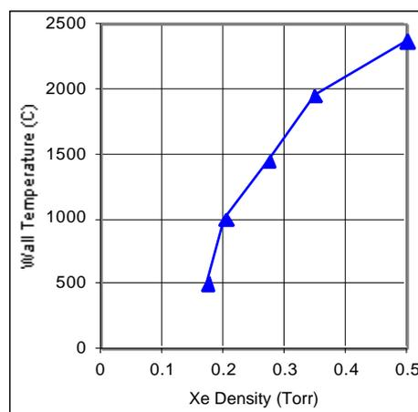
Figure 4 Pre-shot  $T_{\text{wall}}$  at which one C monolayer is vaporized per shot as a function of Xe density for a 6.5 m radius chamber under the ID target spectra.
