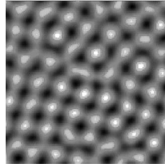
Fig. (5c): Results of numerical solutions for surface deformation patterns in laser-irradiated surfaces [5].
