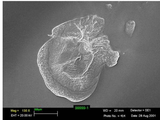
Figure 9. SEM photo of pure Al exposed to one shot at  $180 \text{ J/cm}^2$
