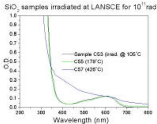
Fig. 1. Results for irradiating fused silica for  $\sim 10^{11}$  rads at the indicated temperature.
