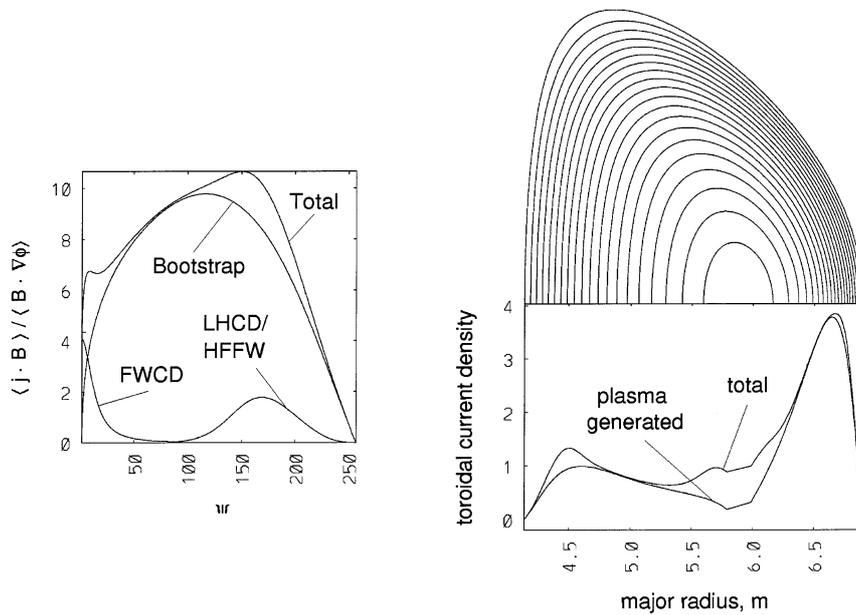
Fig. 2. ARIES-RS reference plasma equilibrium parallel current profile as a function of poloidal flux, the plasma flux surface contours, and toroidal current density as a function of the major radius.
