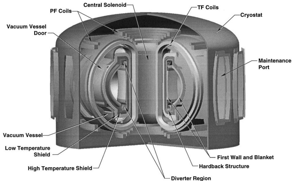
Fig. 3. Cutaway of the ARIES-RS power core.
