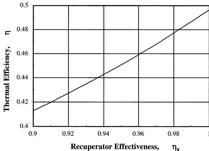
Fig. 2. Influence of recuperator effectiveness on thermal efficiency of power conversion system (all other parameters are listed in Table 1).
