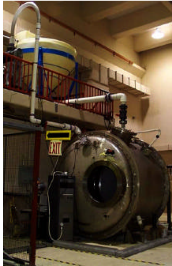
Fig. 1. This UCB facility uses transient flow into a large vacuum vessel to study single jets (currently) and partial-liquid pockets with a few jets (future plans). Water can be used to simulate Flibe jets at 1/2 to 1/4 geometric scale with dimensionless Re , Fr and We numbers matching those in a power plant chamber.
