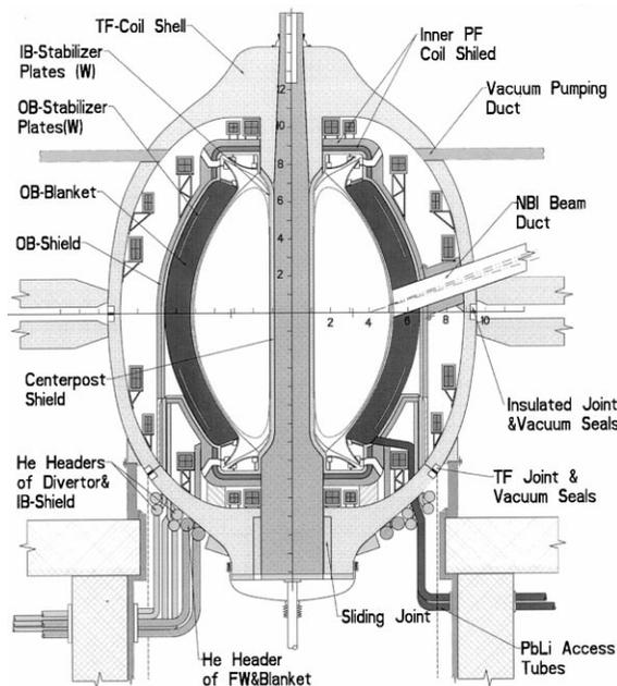
Fig. 1. Elevation view of the ARIES-ST power core.
