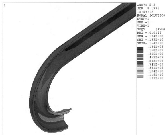
Fig. 5. Thermal plus pressure (12 MPa) stresses in the divertor outer pipe.
