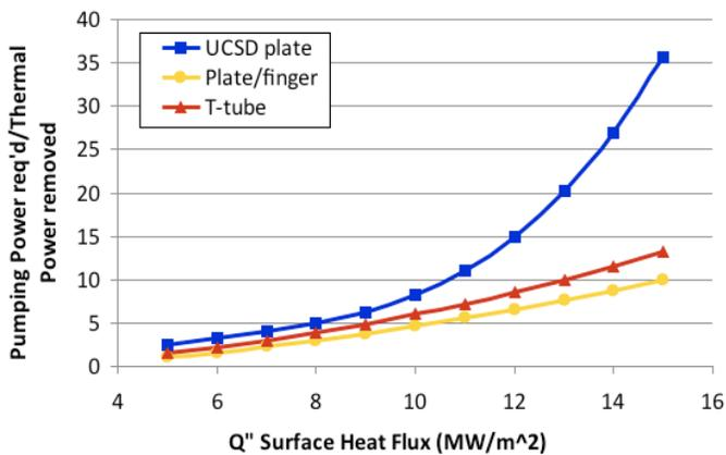
Figure 1. Pumping power correlations for the three helium-cooled December 2010 divertor designs.
