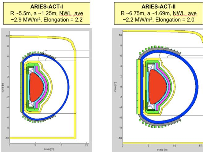
Figure 3. Radial build drawings from the systems code of the aggressive physics ACT-I and the conservative physics ACT-II. The drawings are scaled to the same dimensions for comparison.
