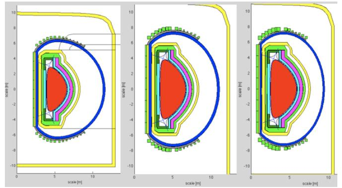
Figure 4. Radial build drawings from the scanning of the aspect ratio. A = 4.0 (left), A = 3.0 (center), A = 2.5 (right). As aspect ratio is reduced from left to right, note decreasing major radius, elongation of TF coil (blue) and increased size of PF coils on top and bottom (green).
