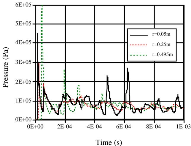
Figure 9. Pressure histories at  $x=0.5\text{ m}$  for the beamline case
