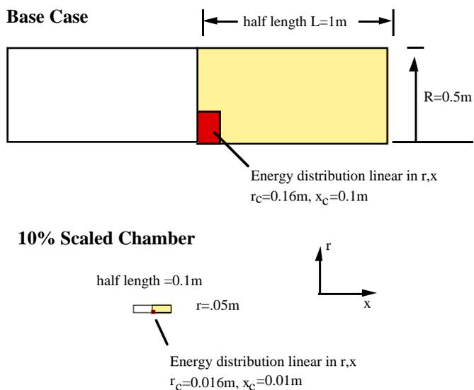
Figure 1. Cylindrical chamber geometry
