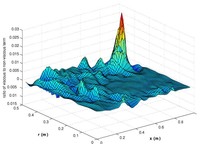
Figure 7. Ratio of viscous to inertial terms for Case I ( $v_x$  in  $x$  momentum equation at 0.9 ms)
