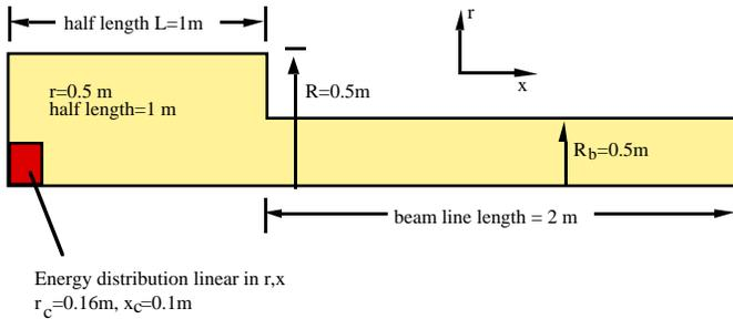
Figure 8. Geometry of cylindrical chamber with beamline
