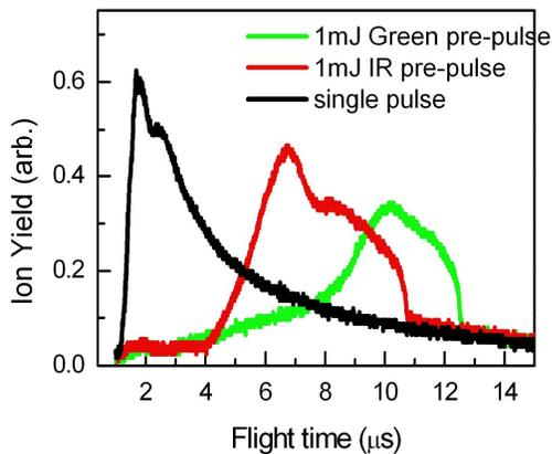
Fig. 3. TOFs from Sn plasma irradiated by dual laser pulses with a pre-pulse with wavelength of IR 1.064 and green  $0.532 \mu\text{m}$ , and single pulse.
