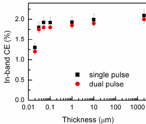
Fig.7. In-band conversion efficiency versus thickness of Sn target, red dot represents experimental data obtained with dual laser pulses, black square is from single pulse.
