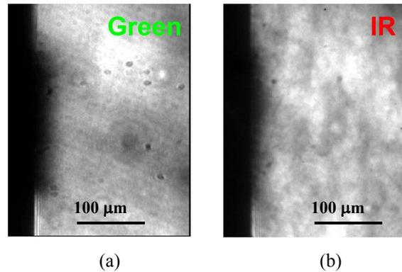
Fig. 4. Shadowgraphs of pre-plume induced by the pre-pulse with wavelengths of (a) IR  $1.064 \mu\text{m}$  and (b) green  $0.532 \mu\text{m}$  respectively.
