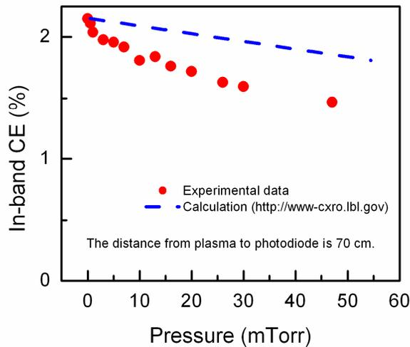
Fig.9. Calculated (blue dashed line) and experimentally measured (red dot) in-band conversion efficiency versus Ar gas pressures.
