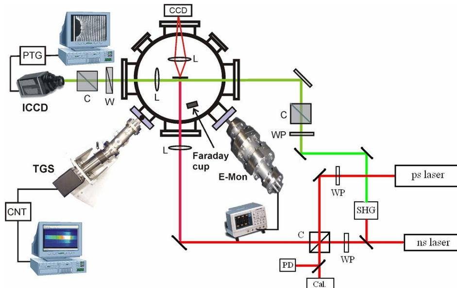
Fig. 1. Experimental arrangement for the generation of EUV light from plasmas irradiated by dual laser pulses. SHG-second harmonic generation, C-cube polarizer, WP-half wave plate, L-lens, PD-photodiode, Cal.-calorimeter, TGS-transmission grating spectrograph, ICCD-intensified CCD camera, W-Wollaston prism.
