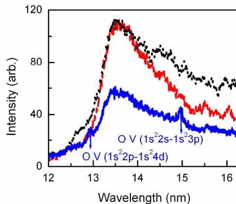
Fig.6. Soft x-ray spectra from Sn plasmas with 1 mm slab (black dot), 30 nm film coated on silicon wafer (red line), and 30 nm film coated on plastic plate (blue line).
