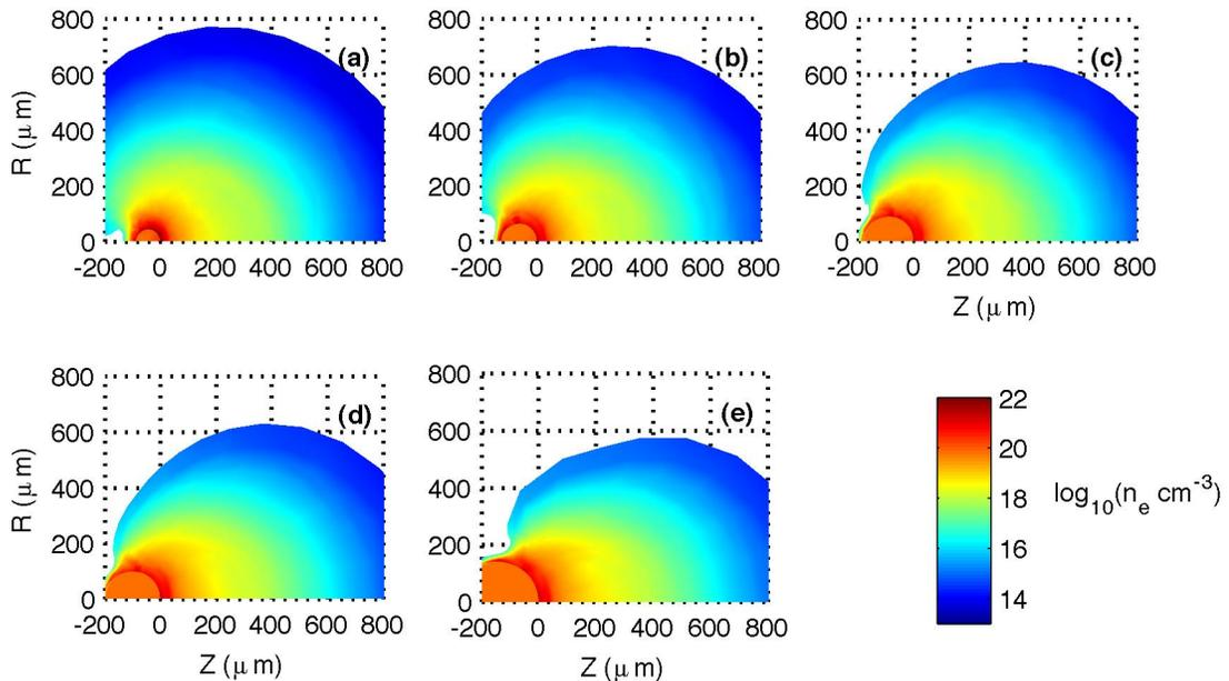
FIG. 3. The electron density at the peak of the laser for SD/FSS ratios of (a)1.13, (b)1.63, (c) 2.25, (d) 2.50 and (e) 3.50. The edge of the spheres are positioned at Z=0.
