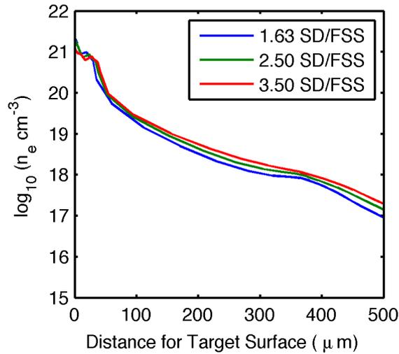
FIG. 4. The electron density along the laser axis at the peak of the laser for SD/FSS ratios of 1.63 (blue), 2.50 (green) and 3.50 (red).
