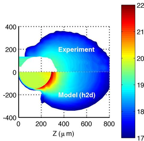
FIG. 1.  $\text{Log}_{10}$  of the electron density at the peak of the laser pulse for a typical experimental (top) and h2d simulation (bottom)  $280\ \mu\text{m}$  diameter sphere. The diagnostic limitation of the experiment is  $10^{17}\text{-}10^{19}\ \text{n}_e\ \text{cm}^{-3}$ .
