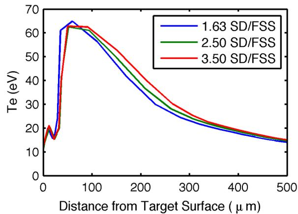
FIG. 7. The electron temperature along the laser axis at the peak of the laser for SD/FSS ratios of 1.63 (blue), 2.50 (green) and 3.50 (red).
