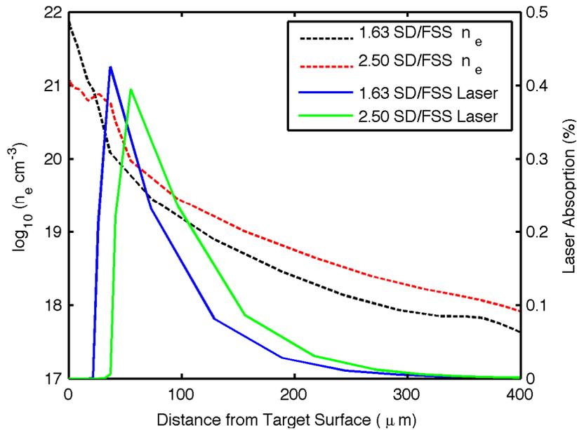
FIG. 5. The laser absorption along the axis at the peak of the laser pulse for SD/FSS ratios of 1.63 (blue) and 2.50 (green). Also plotted is the electron density for SD/FSS ratios of 1.63 (black dashes) and 2.50 (red dashes).
