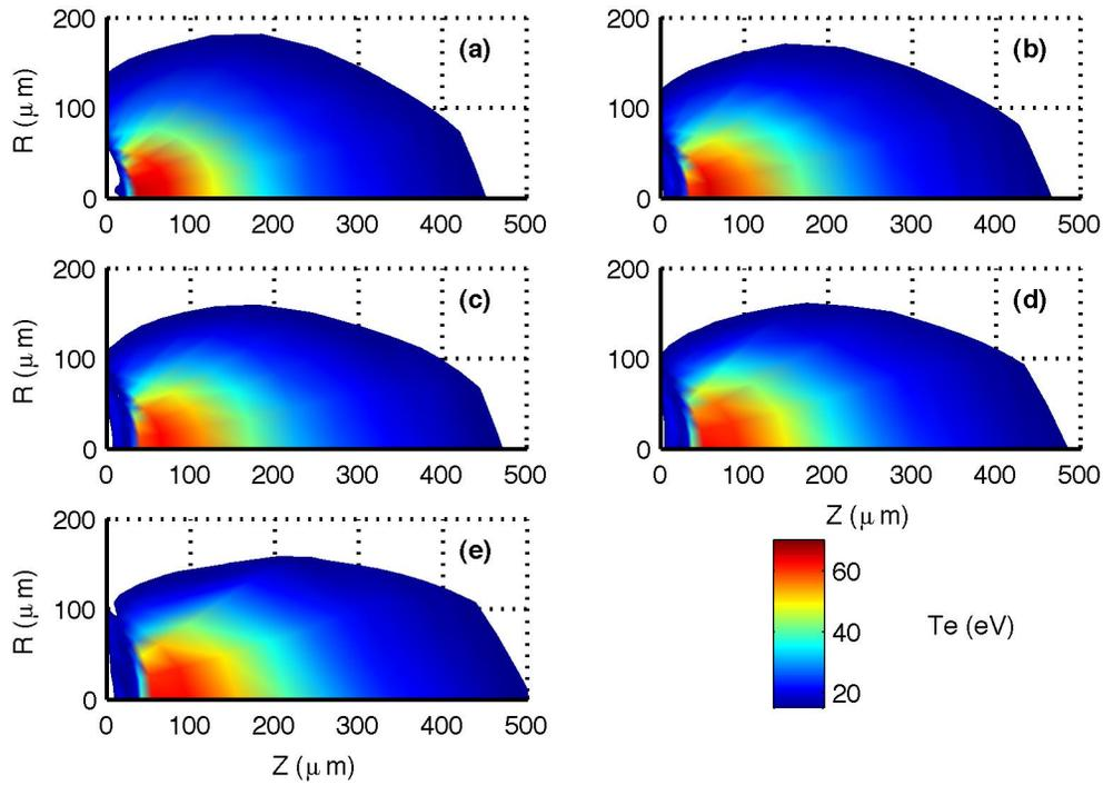
FIG. 6. The electron temperature at the peak of the laser for SD/FSS ratios of (a) 1.13, (b) 1.63, (c) 2.25, (d) 2.50 and (e) 3.50. The edge of the spheres are positioned at  $Z=0$ .
