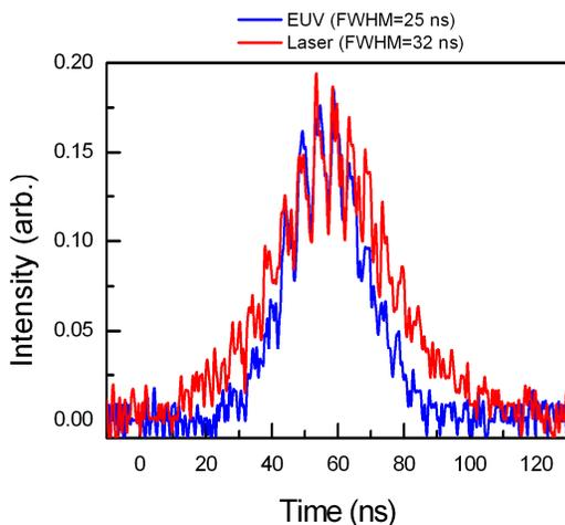
Figure 10. Waveforms of 32 ns laser pulse and its EUV emission
