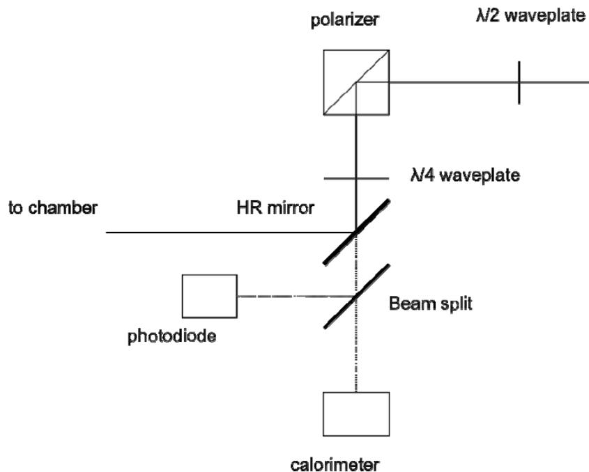
Figure 3. Experimental arrangement for the interaction of long duration laser pulse with Sn plasma
