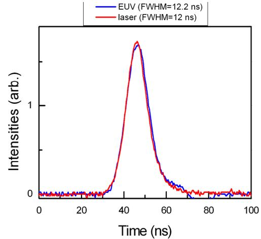
Figure 9. Waveforms of 12 ns laser pulse and its EUV emission
