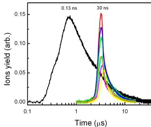
Figure 11. Time of flight of ions from Sn plasmas irradiated with 0.13 and 30 ns laser pulses
