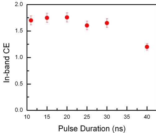
Figure 4. In-band CE as a function of laser pulse durations
