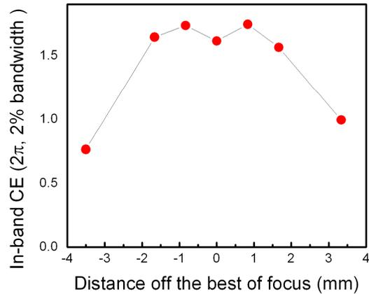
Figure 5. In-band CE from Sn plasma irradiated with 0.13 ns laser pulse as a function of lens position
