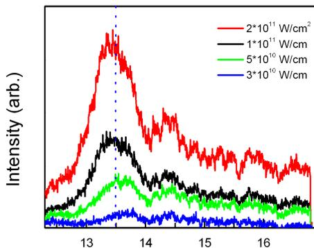
Figure 6. Soft x-ray spectra of Sn plasma irradiated with 30 ns laser pulse with various laser intensities
