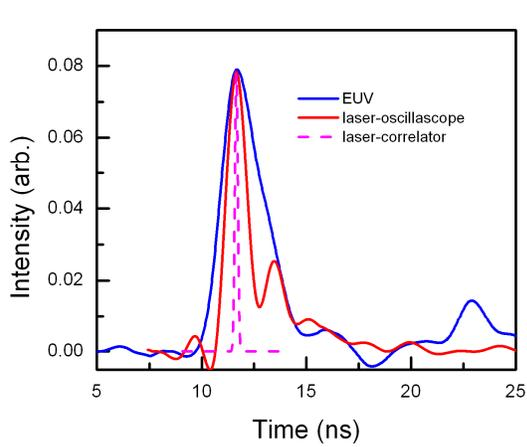
Figure 8. Waveforms of 0.13 ns laser pulse and its EUV emission
