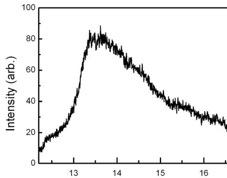
Figure 7. Soft x-ray spectrum of Sn plasma irradiated with a 0.13 ns laser pulse
