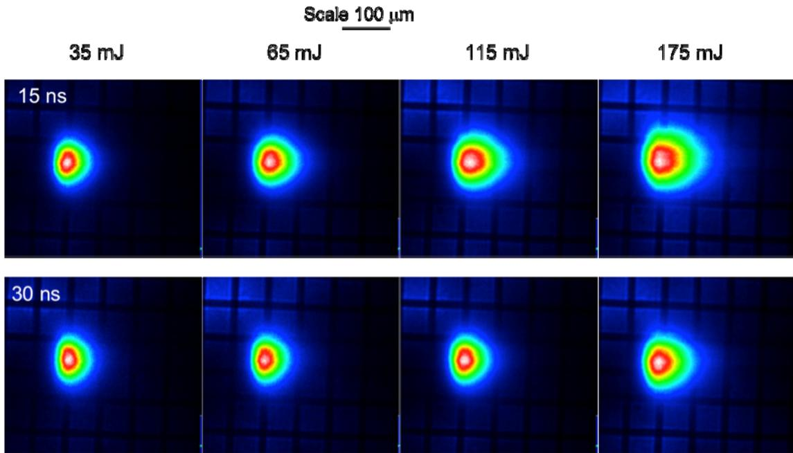
Figure 12. In-band EUV images of Sn plasma irradiated with laser with pulse durations of 15 and 30 ns with various pulse energy
