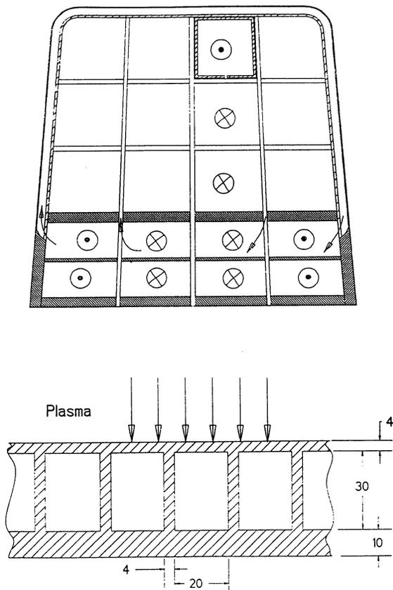
Fig. 4. Dual coolant first wall blanket configuration.
