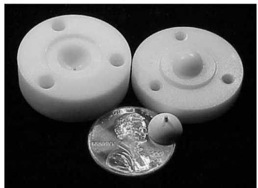
Fig. 3. Injection-molded 4 mm diameter hemispherical shell with a 400 μm wall.
