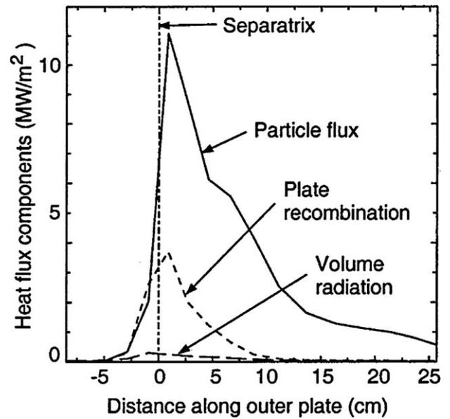
Fig. 7. Heat flux profile for ARIES-AT.
