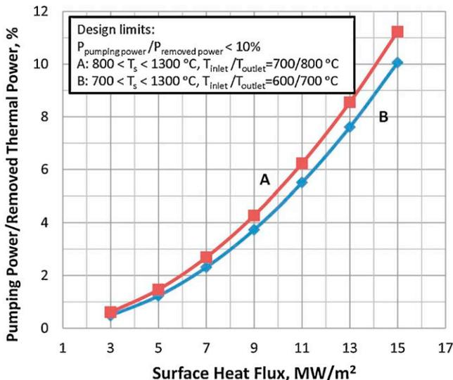
Fig. 6. Parametric studies of the finger divertor showing the allowable surface heat flux constrained by the operating temperature and pumping power.
