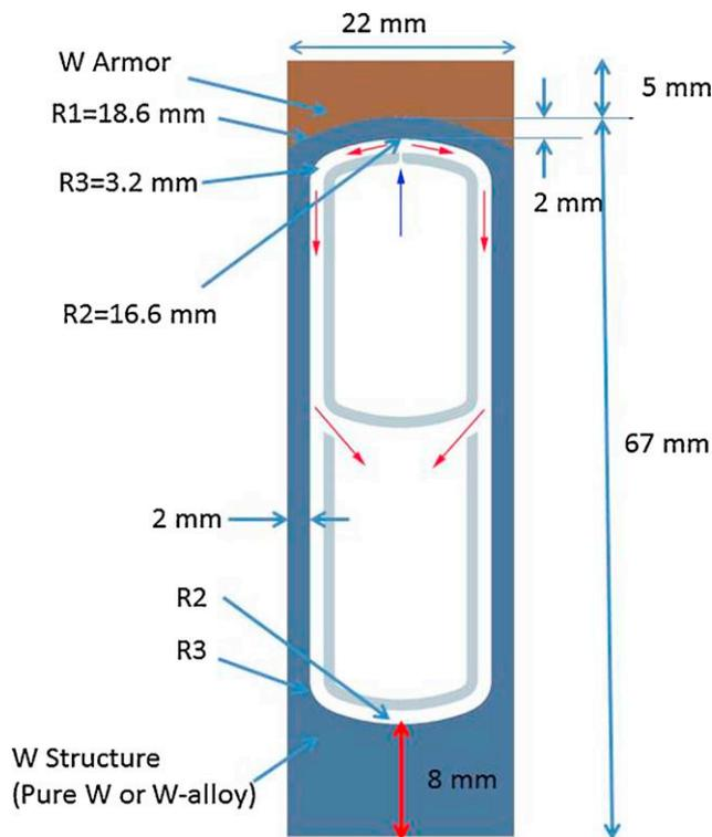
Fig. 1. Schematic of the plate-type divertor.
