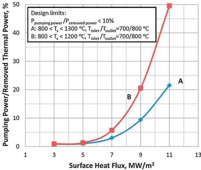
Fig. 5. Parametric studies of the plate divertor showing the allowable heat flux constrained by the operating temperature and the pumping power.
