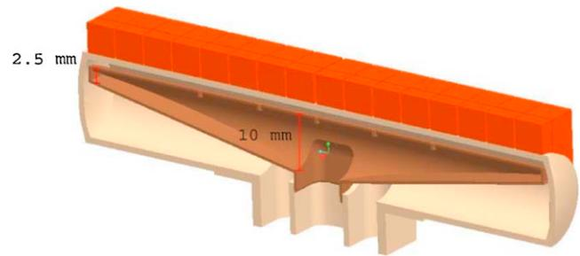
Fig. 2. Schematic of the T-tube divertor.
