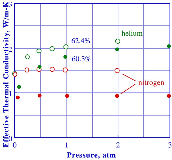
Figure 5. Thermal conductivity vs. gas pressure in 0.1-mm Al beds (with packing fractions 57.4 and 58.8%) with He and N<sub>2</sub> fill gas. Open circles denote previously reported data.
