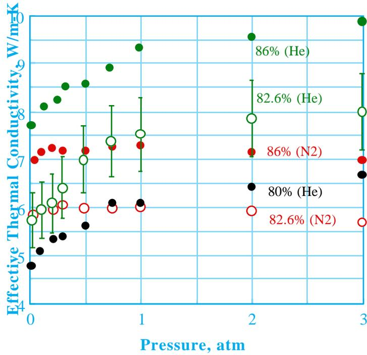
Figure 7. Thermal conductivity vs. gas pressure in 0.1+4.3-mm Al binary beds with He fill gas and several packing fractions.
