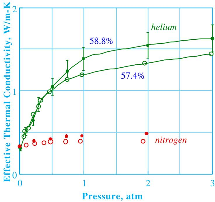
Figure 6. Thermal conductivity vs. gas pressure in 0.5+4.3-mm Al binary beds with He and N<sub>2</sub> gas and several packing fractions. Open circles denote He and closed circles denote N<sub>2</sub>.
