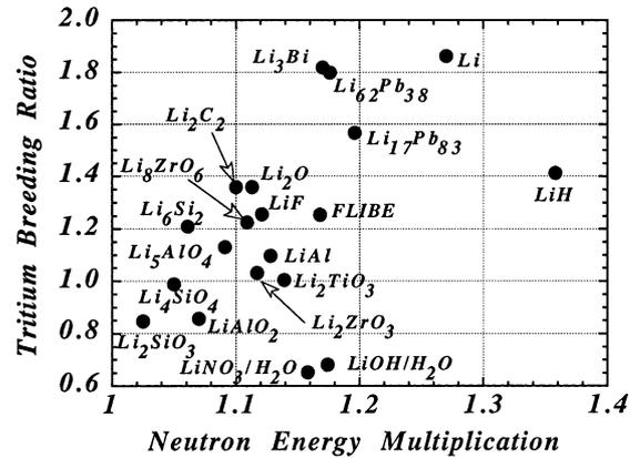
Fig. 3. Tritium breeding ratio versus neutron energy multiplication for candidate breeders (100% dense at room temperature).
