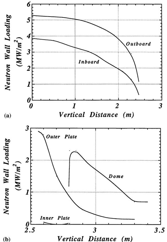
Fig. 2. Poloidal variation of neutron wall loading.
