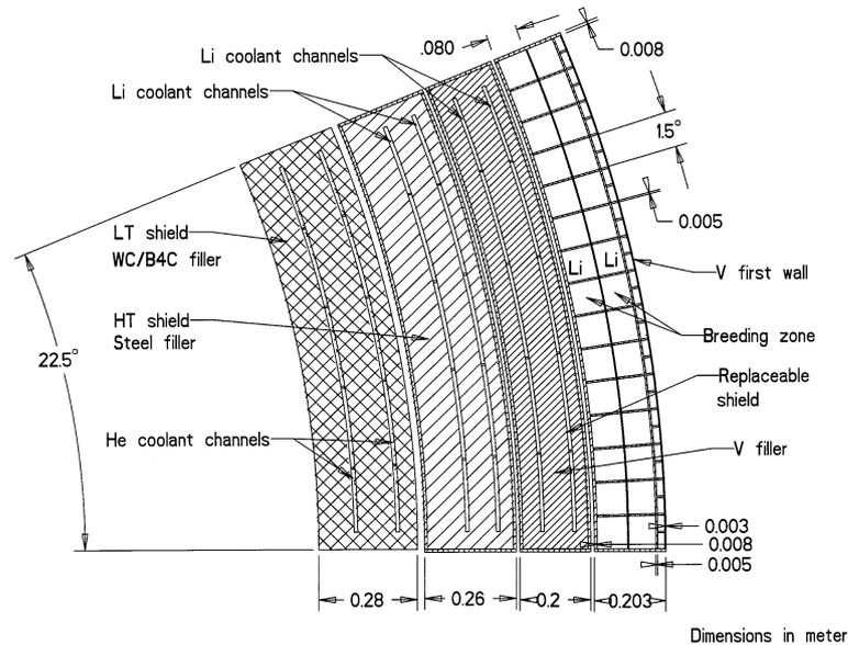
Fig. 7. Cross section of inboard blanket and shield.
