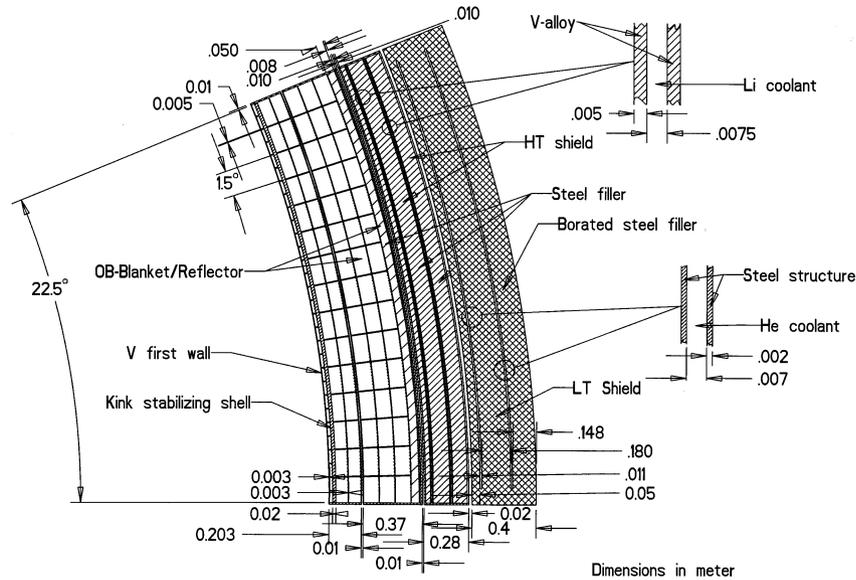
Fig. 8. Cross section of outboard blanket and shield.
