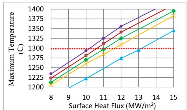
Fig. 5. Maximum temperature of WL10 outer tube vs. surface heat flux. Legend provided in Table III.
