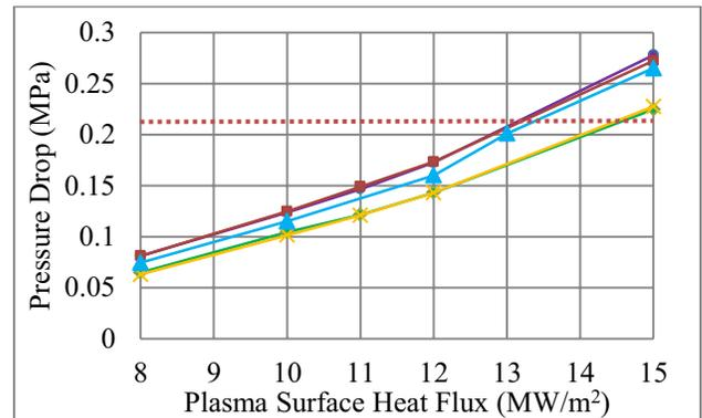
Fig. 4. Pressure drop vs. surface heat flux. Legend provided in Table III.
