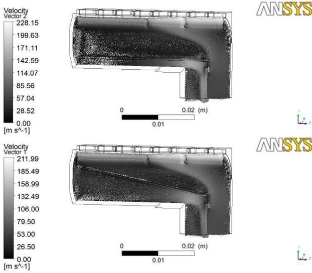
Fig. 3 Velocity vector comparison of the tapered and non-tapered cartridge with all other variables kept constant.
