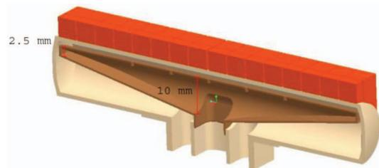
Fig. 2. Modified T-tube design with cartridge tapered from 10 to 2.5 mm. All other dimensions remain the same.
