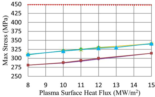
Fig. 6. Equivalent von-mises stress of WL10 outer tube vs. surface heat flux. Legend provided in Table III.
