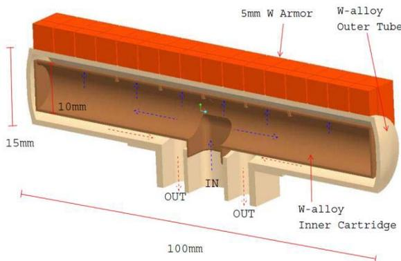
Fig. 1. Original T-tube design with non-tapered cartridge (half cross section).
