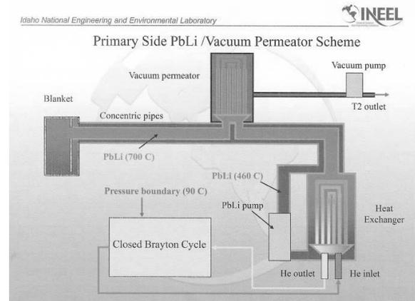
Fig. 7. : Primary loop system with permeator
