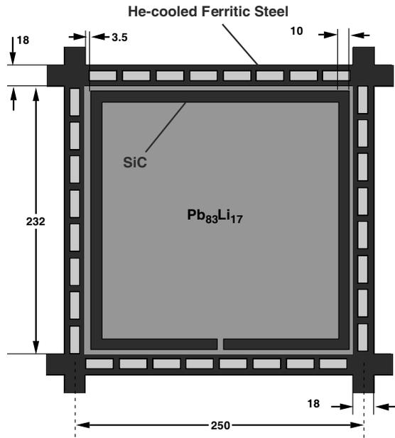
Fig. 3. Configuration of a breeding cell [9]
