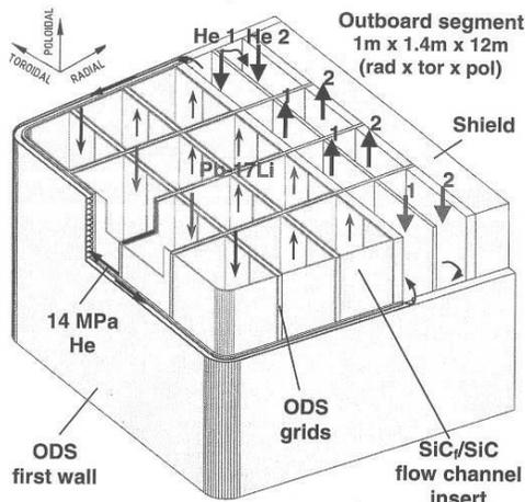
Fig. 4. Isometric view of an outboard blanket segment [11]
