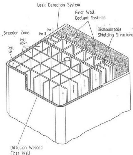
Fig. 2. Perspective view of an outboard blanket segment [7]
