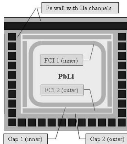
Fig. 8: Principle of nested flow channel inserts [22]
