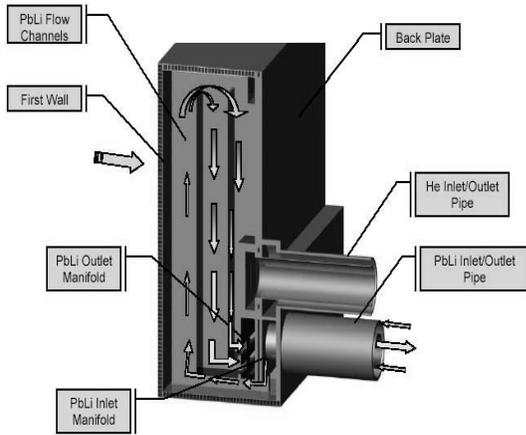
Fig. 5 DCLL blanket configuration with PbLi flow path [20]
