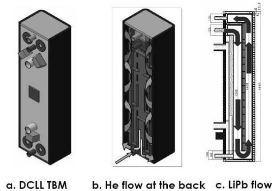
Fig. 6 DCLL ITER TBM module schematics
