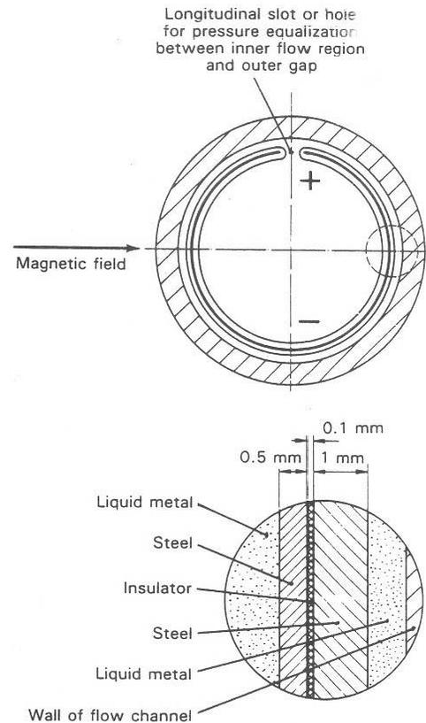
Fig. 1. Principle of Sandwich Flow Channel Insert [5]
