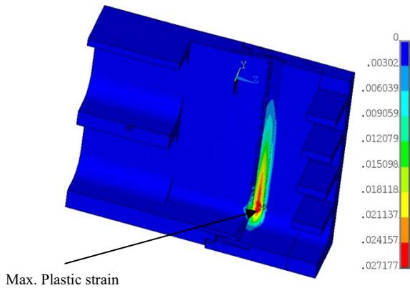
Figure 12. Maximum plastic strain in the full 3-D model
