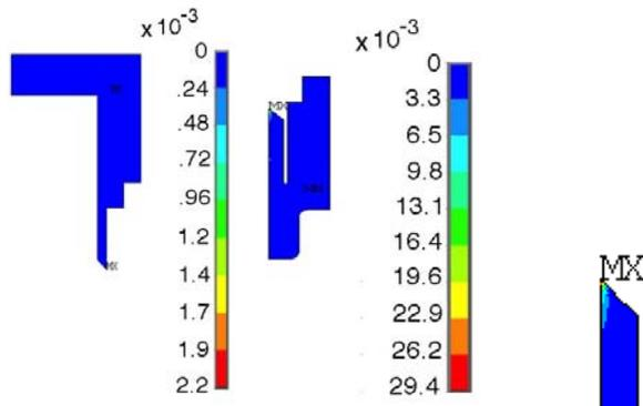
Figure 7. Maximum plastic strain in the ODS steel (left) and Ta (right) after the first warm shutdown
