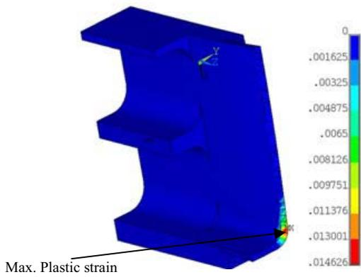
Figure 13. Maximum plastic strain highlighting the ODS steel
