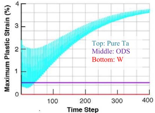
Figure 10. Results of plastic strain with Ta2.5%W for 100 cycles during cold shutdown
