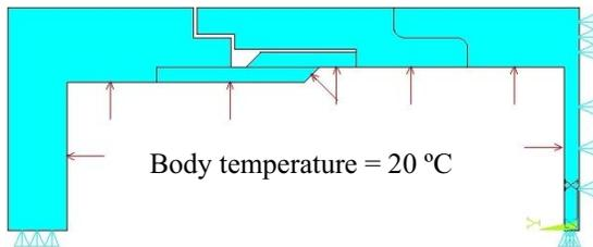
Figure 5. Divertor plate configuration with constraints ( $U_y=0$  at right, and  $U_x=0$  at the bottom), pressure (inner arrows), and body temperature.
