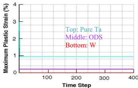
Figure 8. Results of plastic strain for 100 cycles during warm shutdown
