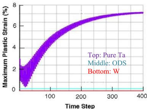
Figure 9. Results of plastic strain for 100 cycles during cold shutdown.
