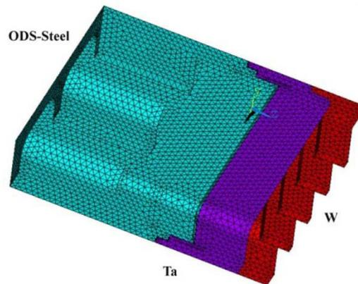
Figure 11. 3D configuration showing 3 materials and the mesh
