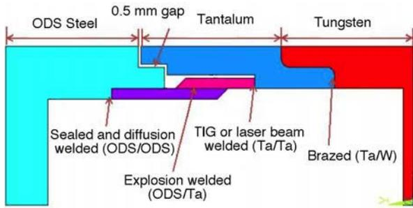
Figure 1. 2-D divertor joint showing materials, geometry, and bonding process.
