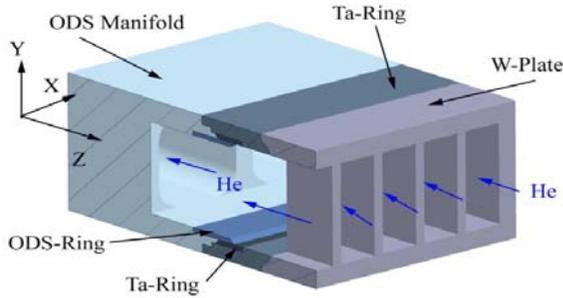
Figure 4. 3-D divertor model with 2-D cross section and He as a coolant
