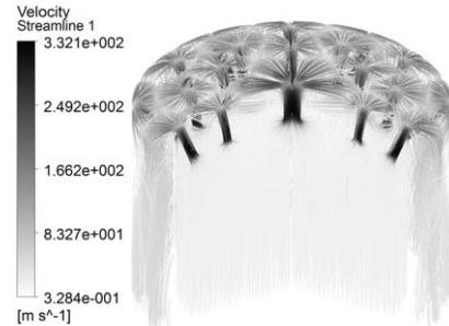
Fig. 6. Velocity distribution in the channel illustrating the jet flow to cool the heated zone
