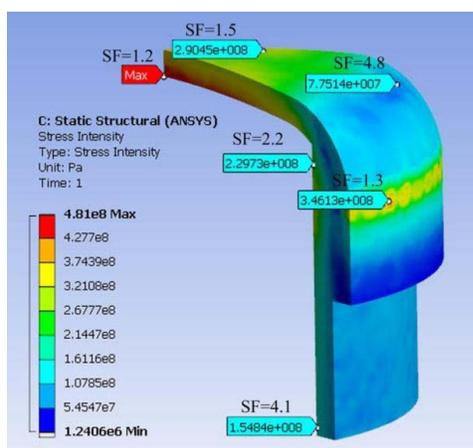
Fig. 8. Combined stress (primary + secondary) distribution after stress relaxation
