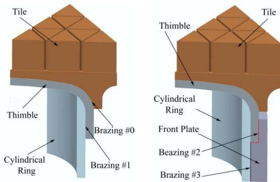
Fig. 2. Fabrication of the finger unit
