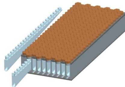
Fig. 4. The divertor target with inserted cooling cartridges
