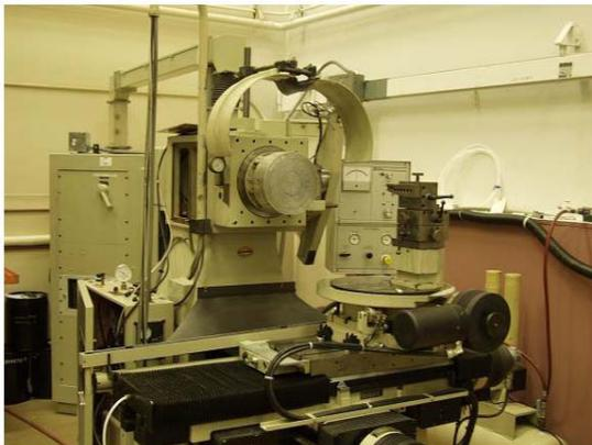
Figure 2. Diamond Point Turning Machine.
