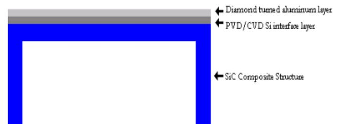
Figure 1. Current Design Concept for Al/SiC.
