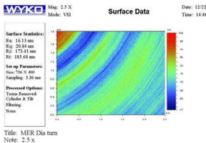
**Figure 8. Microroughness of a Polished Diamond Turned Al Disk.**
