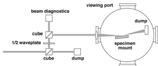
**Figure 4. Experimental Setup for Mirror Damage Studies.**
