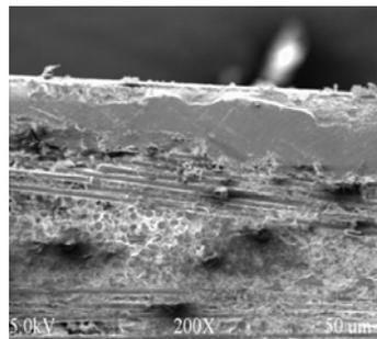
**Figure 6. Aluminum Foil Diffusion Bonded to SiC Structure.**
