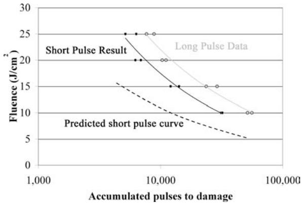
Fig. 12. Short pulse damage fluence data compared with prediction based on thermal diffusion
