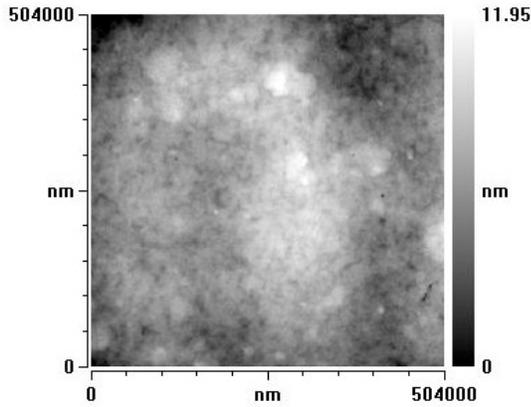
Fig. 8. Surface profilometry for a CMP polished mirror
