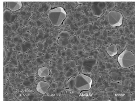
Fig. 9. SEM image of an alloy mirror prior to surface finishing
