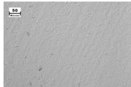
Fig. 11. Damage to Alumiplate mirror at high cycle count.
