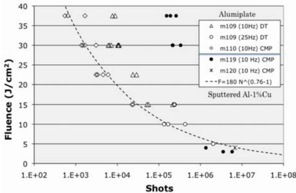
Fig. 10. Long pulse damage fluence data comparing Alumiplate and sputtered alloy mirrors.
