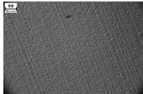
Fig. 6. Microscopy of a diamond-turned alumiplate mirror
