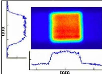
Fig. 4. Homogenized beam profile
