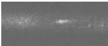
Fig. 5. Vision system image prior to automated shutdown. A HeNe laser backlighter is used to enhance the signal.
