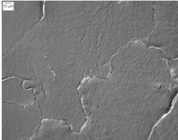
Fig. 1. Mechanisms of laser-induced damage in metal mirrors: grain boundary rotation
