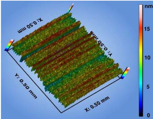
Fig. 7. 2D surface profilometry for a diamond-turned Alumiplate mirror
