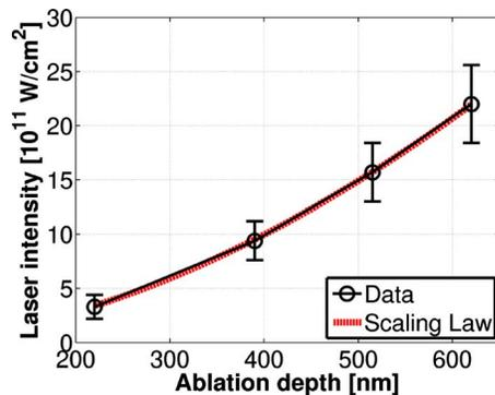
FIG. 6. (Color online) Variation of ablation depth with laser intensity, and comparison with a (5/9)th power fit.
