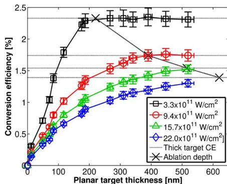
FIG. 2. (Color online) CE as a function of planar target thickness at each of the four nominal laser intensities.
