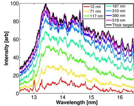
FIG. 3. (Color online) Evolution of the EUV spectrum at a laser intensity of  $15.7 \pm 2.7 [10^{11} \text{ W/cm}^2]$  as the target thickness is increased.
