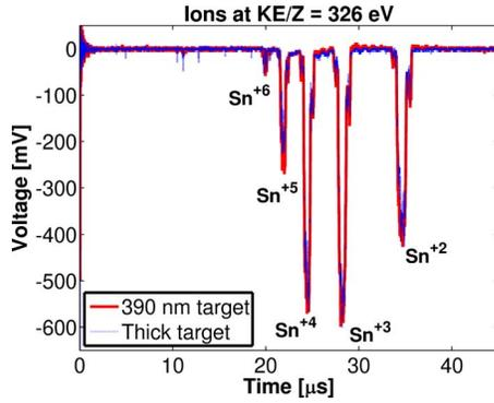
FIG. 5. (Color online) Time-of-flight data generated by the electrostatic ion energy analyzer at a laser intensity of  $9.4 \pm 1.8$  [ $10^{11}$  W/cm $^2$ ] for the thick target and a 390 nm target. The signal levels are identical in both waveforms, indicating the ablation depth was reached.
