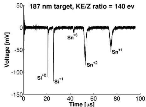
FIG. 4. Time-of-flight data generated by the electrostatic ion energy analyzer at a laser intensity of  $9.4 \pm 1.8 [10^{11} \text{ W/cm}^2]$  using a 187 nm thick target. Each negative-going peak in the waveform represents the arrival of an ion species at the output of the probe meeting the filter criterion ( $KE/Z=140 \text{ eV}$ ).
