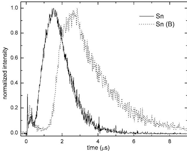
FIG. 1. Typical TOF profiles of Sn species recorded at a distance of 13 mm from the target surface in the presence (slowed one) and absence (faster profile) of magnetic field.
