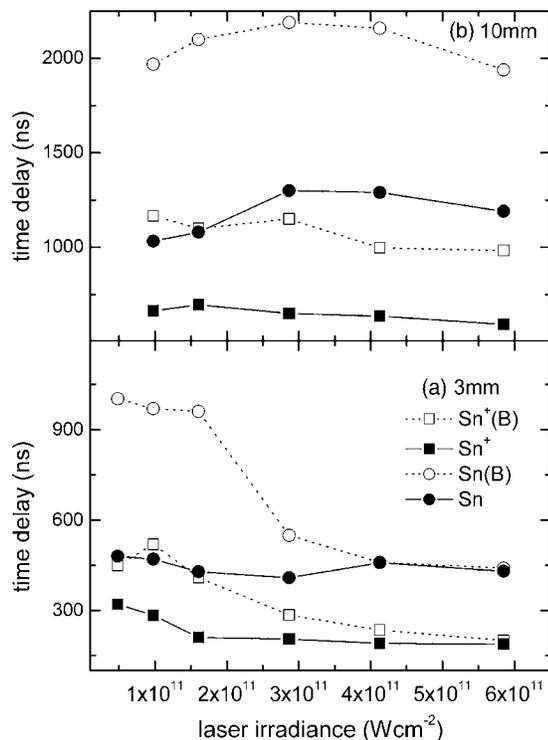
FIG. 3. The dependence on laser irradiance of the arrival time for Sn (●,○) and Sn<sup>+</sup> (■,□) species is given for  $B$  (hollow symbols, dot lines) and with out  $B$  (filled symbols, solid lines) for different distance from the target surface [(a) 3 mm and (b) 10 mm].
