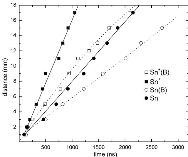
FIG. 2. The  $R-t$  (position-time) for the Sn (●,○) and  $\text{Sn}^+$  (■,□) species in the presence (hollow symbols, dot lines) and absence (filled symbols, solid lines) of magnetic field is given. The laser irradiance used is  $300 \text{ GW/cm}^2$ .
