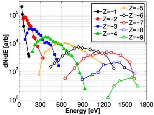
FIG. 4. (Color online) Charge-state resolved ion energy distribution measured at a distance of 100 cm from a Sn target irradiated by a CO<sub>2</sub> laser with parameters described in Table I.
