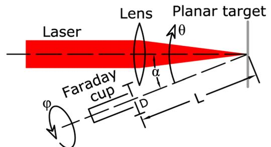
FIG. 1. (Color online) Experimental arrangement for measurement of the critical distance. A focused laser irradiates a planar target at normal incidence. A faraday cup with aperture diameter  $D$  is installed at an angle  $\alpha$  to the target normal and can be translated distances  $L$  along the path of plasma expansion. A spherical coordinate system with zenith angle  $\theta$  and azimuthal angle  $\phi$  with respect to the faraday cup translation axis is superimposed.
