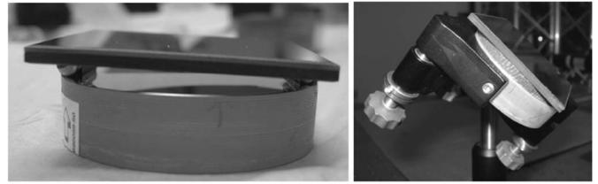
Fig. 5. Simulated monolithic wedged dichroic mirror (5-cm diameter).
