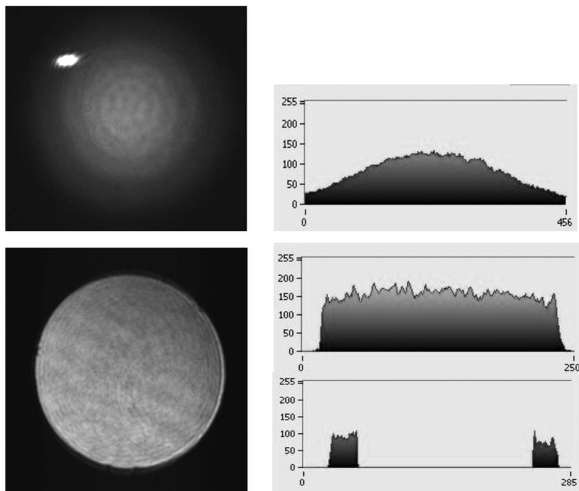
Fig. 6. (Top) Prior Gaussian driver beam with lineout. (Bottom) New flat-top driver beam with lineout of the beam and the target occluding the beam.
