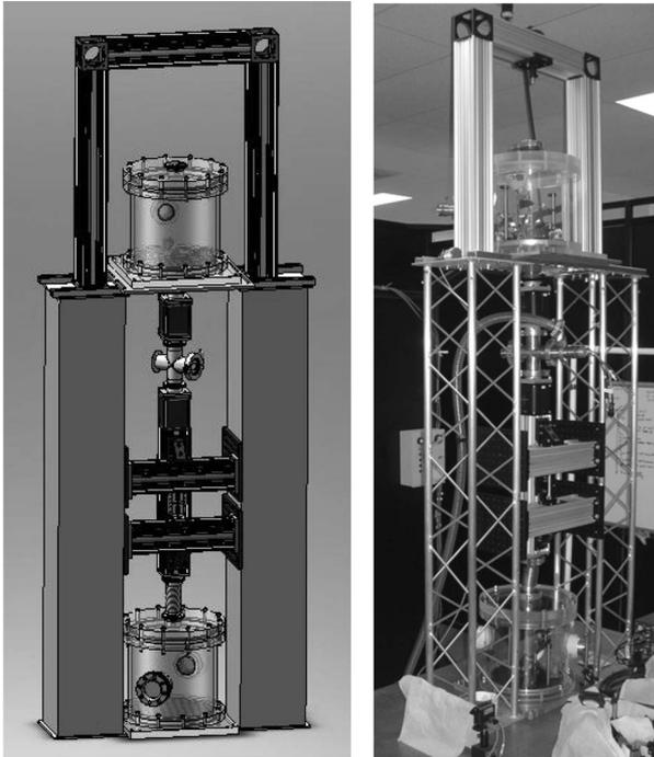
Fig. 4. Drop tower ( $\sim 2$  m tall) with upper and lower vacuum chambers. (Left) CAD drawing and (right) full assembly in the lab.
