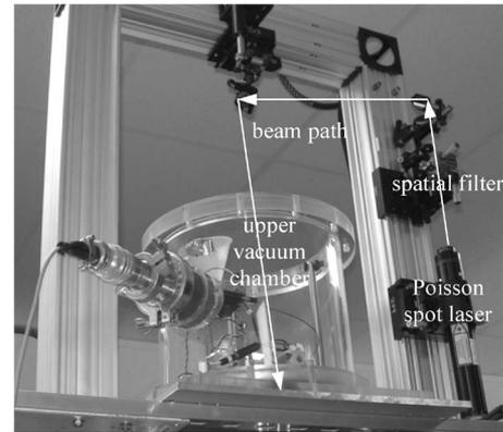
Fig. 3. Upper vacuum chamber on top of a support tower showing Poisson spot illumination beam being assembled and directed downward.
