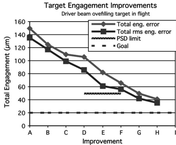
Fig. 2. Stepwise improvement graph with effect on the overall target engagement results. (A) Initial setup, 4:1 magnification, and defocused GR. (B) Focused GR. (C) Focused GR and small aperture. (D) 1:1 magnification. (E) 1:1 magnification, improved steering calibration. (F) Glint camera that replaces position-sensitive diode (PSD). (G) Stable beam splitter and small delta steering. (H) Vacuum chamber. (I) (Anticipated) Thermal drift and electrical noise eliminated.
