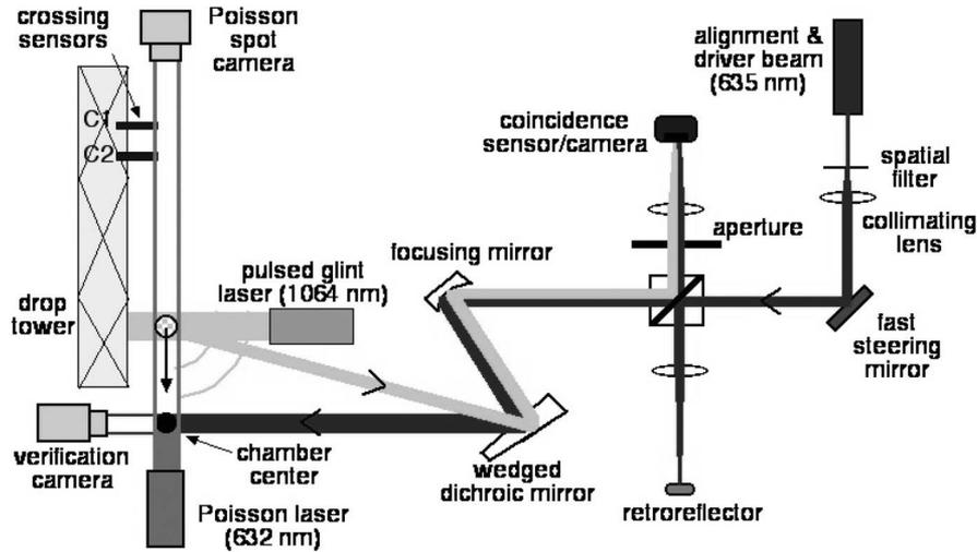
Fig. 1. Schematic of integrated target tracking and engagement demonstration. Focusing mirror to the chamber center is 2 m; drop tower is ~2 m tall (figure not to scale).
