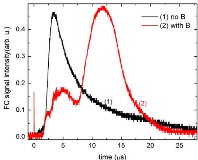
FIGURE 8 The Faraday cup ion signal recorded in the presence and absence of a magnetic field
