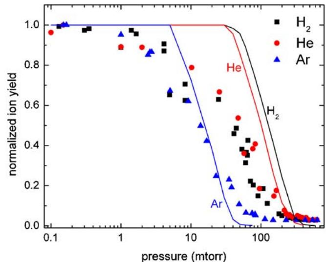
FIGURE 6 Integrated ion yield obtained from Faraday cup TOF ion data at different gas pressure levels of argon, helium and hydrogen. The solid curves correspond to ions yield obtained from SRIM
