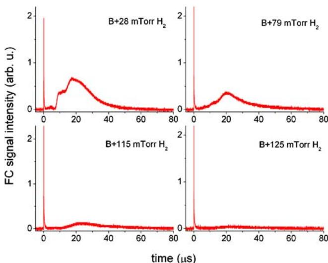
FIGURE 9 Faraday cup ions signal in the combined effect of a magnetic field and ambient gas
