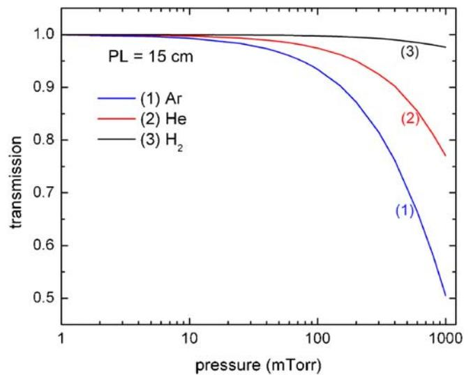
**FIGURE 1** Transmission of 13.5 nm radiation at different argon and helium pressures is given for a path length of 15 cm
