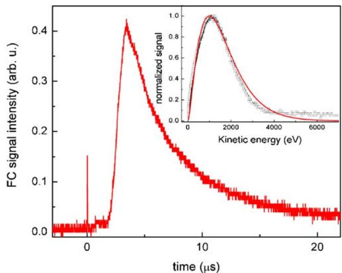
FIGURE 4 TOF of ions recorded using a Faraday cup placed at a distance  $\sim 15$  cm from the target surface for plume expansion into vacuum. The kinetic distribution of the tin ions obtained from TOF signal in vacuum is given in the inset. The solid line represents the SMB fit and points represent experimental data points
