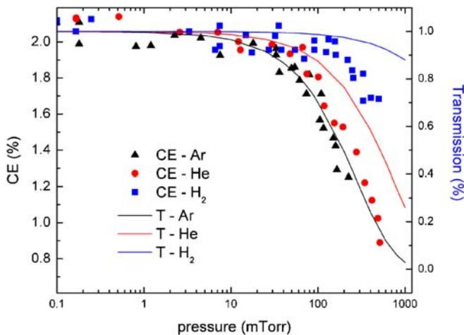
FIGURE 7 The variation with CE with buffer pressure is given. The symbols represent the experimental data points and the curves give the 13.5 nm transmission (T) at different gas pressures for a path length of 78 cm
