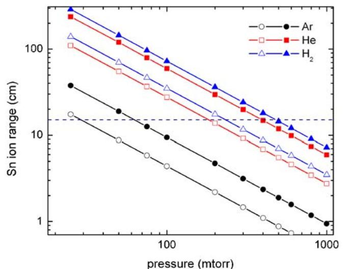
**FIGURE 2** The SRIM estimate of the flight range of tin ions with different values of initial energies propagating into an ambient gas is shown. The hollow symbols correspond to a starting energy of 1 keV and the darkened symbols are for 5 keV. The dashed line in the center corresponds to the Faraday cup position (15 cm)
