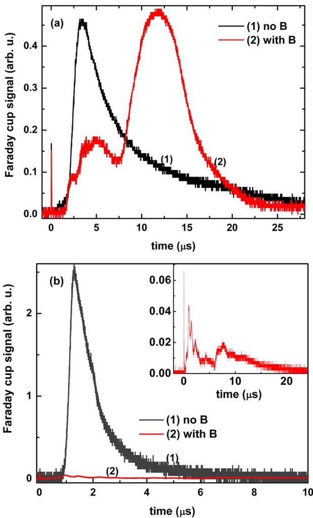
Fig. 3. (Color online) Typical ion time-of-flight signals recorded for (a) full density and (b) 0.5% density Sn in the presence and in the absence of a magnetic field. A magnified version of the time-of-flight profile obtained from 0.5% Sn in the presence of a magnetic field is given in the inset of (b).
