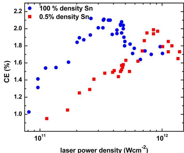
Fig. 2. (Color online) Estimated CE for a full-density Sn and a 0.5% Sn-doped foam target at various laser intensities.
