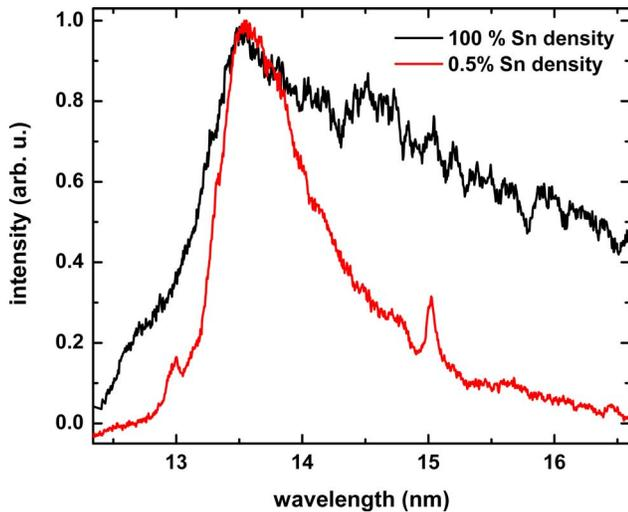
Fig. 1. (Color online) UTA obtained from full-density and 0.5% density Sn. The UTA spectrum from Sn-doped foam targets showed distinct narrowing. Both spectra were recorded with a laser intensity of  $4 \times 10^{11} \text{ W cm}^{-2}$ .
