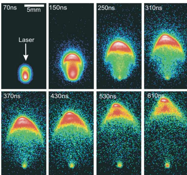
**Figure 1.** The evolution of visible emission from an aluminium plume recorded using an ICCD camera (gating time 2 ns). The laser power density used was  $3 \text{ GW cm}^{-2}$  and background pressure was 150 mTorr. All the images are normalized to their maximum intensity.
