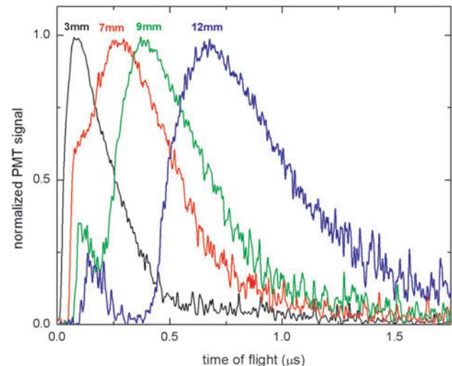
**Figure 3.** Intensity variation of spectral emission with time for  $\text{Al}^+$  species (358.6 nm) recorded at different distance from the target surface. The laser power density was  $3 \text{ GW cm}^{-2}$  and the background air pressure was 150 mTorr for these measurements.
