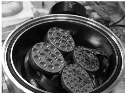
Fig. 3. Planetary-rotating stage with cups for coating shells and tilted to make shells roll when coating.
