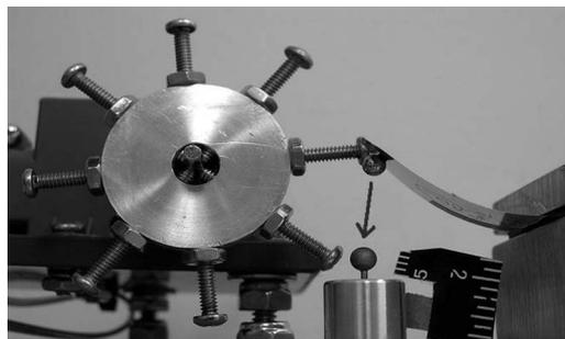
Fig. 6. Picture of automated tapping mechanism.
