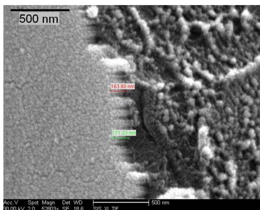
Fig. 4. Example SEM image showing coating thickness measurement technique on coated spherical shells.
