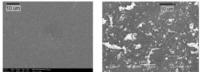
Fig. 1. SEM images of coated surfaces before fluidizing on the left and after fluidizing for 16 h on the right.
