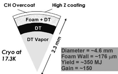
Fig. 2. Section view of a typical HAPL target. [7].
