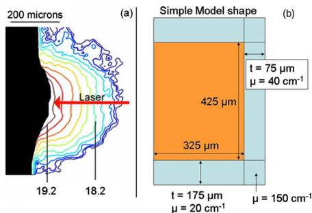
FIG. 2. (Color online) (a)  $\text{Log}_{10}$  of the plasma density at the peak of the laser pulse. The arrow indicates the pump laser direction. (b) Modeled plasma shape with the emitting plasma (orange) and the surrounding plasma (blue).
