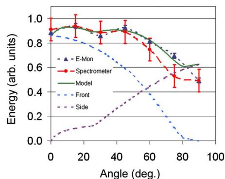
FIG. 1. (Color online) EUV emission at various angles measured with the E-Mon (blue dashed line), TGS for comparison (red dashed line), and modeled values (green line) with front and side surface components (light blue and purple dashed lines). TGS and calculated values are scaled to match the E-Mon measurements.
