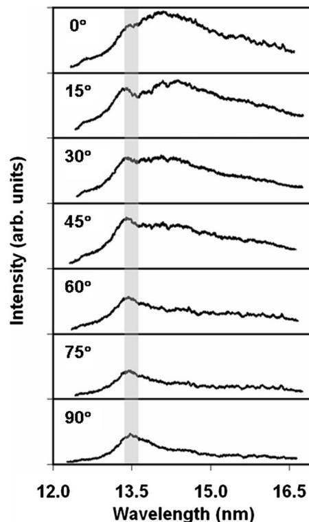
FIG. 3. Typical soft x-ray spectra measured at each angle with the 2% in-band spectral range shaded.
